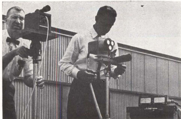
EXPERIMENTAL transmitter (left) and receiver (right) are manually aimed. Servo coupling would make operation automatic
