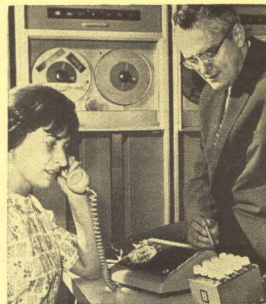
KEYBOARD (lower right) transmits inquiries over commercial telephone lines to a modified Honeywell computer, which processes them and responds with a voice answer. The system can handle as many as 28 different inquiry routines
