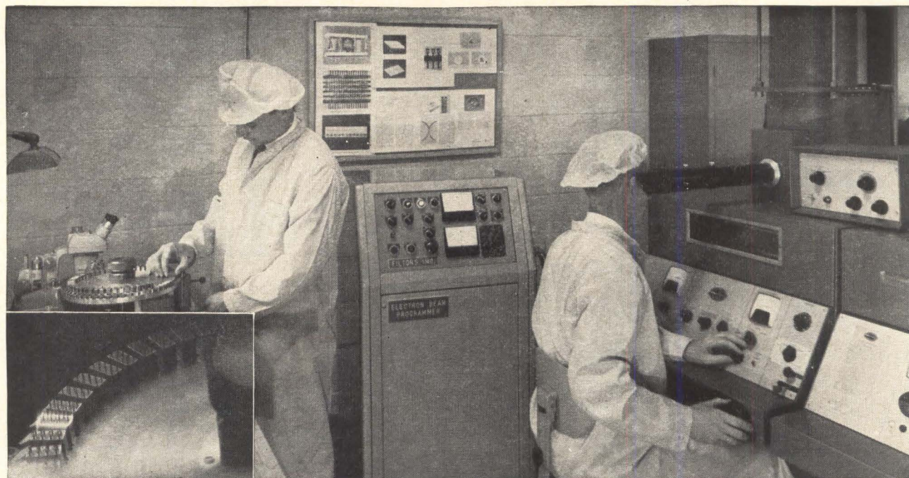
POSITIONING FIXTURE is loaded with relays during welding of other relays. Inset shows multi-exposure photo of beam-impingement traverse on relay. Beam travel is controlled by specially-designed programmer unit in center
