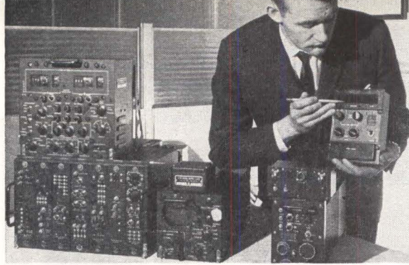
ENGINEER Robert Hudelson points out readout display on mockup of ARN-76 control indicator. Below are antenna coupler and receiver, at left is Sperry's operational airborne Loran-C receiver weighing more than 100 pounds
