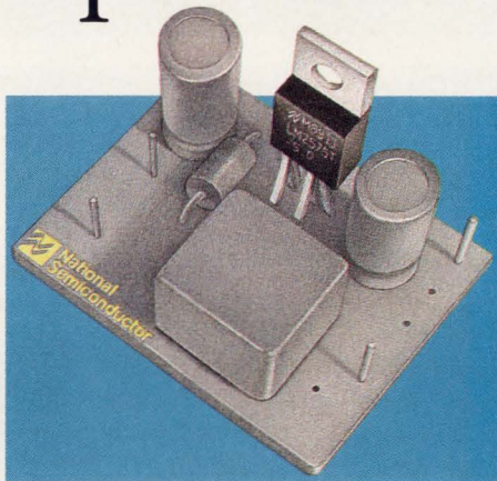
National's LM2575 Simple Switcher requires just four external components.
