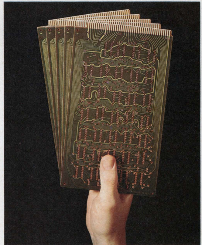
The advantages of additive PC processing include no copper undercutting and more efficient copper use.
