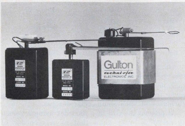
Galvanometers with position servos: The center unit uses pressurized ink while the two others write with indirectly-heated stylus. The thermal units, though, usually require the use of heat sensitive chart paper.
