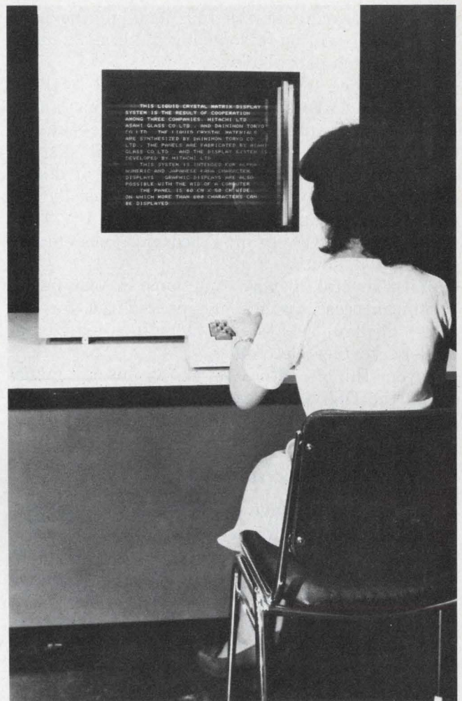
The world's largest LCD system can display more than 600 alphanumeric characters. Produced by Hitachi, it may one day compete with plasma panels and CRTs for computer-terminal applications.
