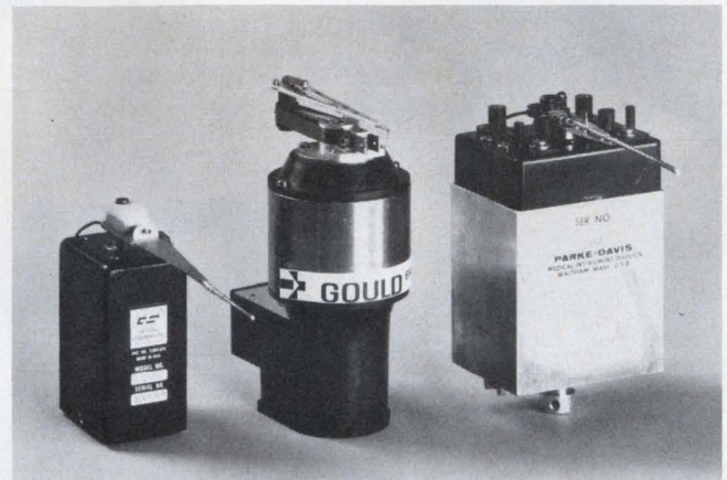
Velocity-feedback galvanometers of equivalent performance: The two larger units are intended for EKG recording with heated stylii, while the smaller unit uses ink for recording EEGs.
