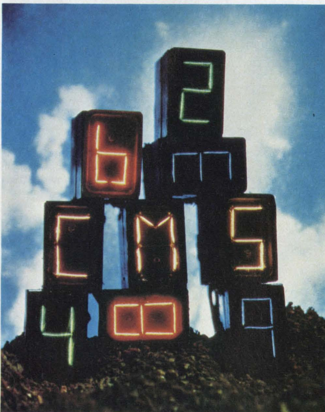
Incandescent displays are best for high brightness. Full color capability is another big plus for incandescents. These CM5 devices from Chicago Miniature Lamp are said to last 100,000 hours.
