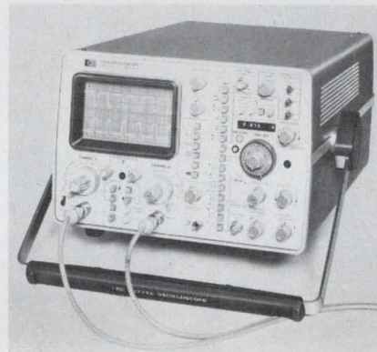
Microprocessors are sure to pop up in more and more instruments, as one did in this Hewlett-Packard calculating scope—the 1722A.
