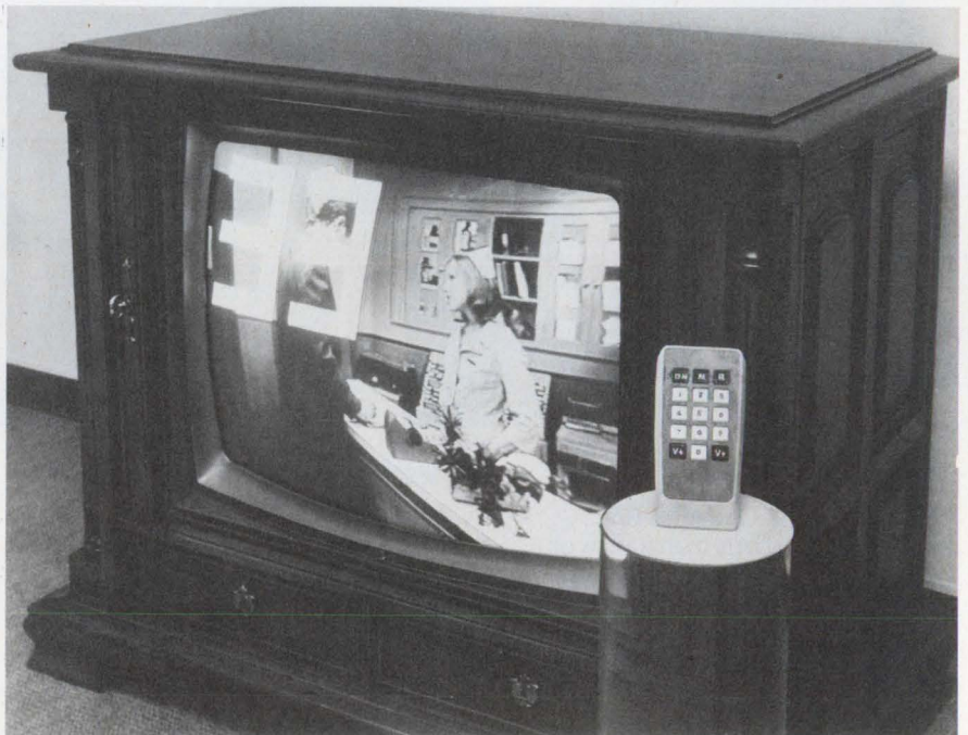
The first all-electronic tuning system with random selection of all 82 TV channels is the Magnavox Star system. Selected channels are briefly shown.
