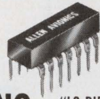
"LC DIP" World's Smallest Dual-in-Line 14 Pin Tapped Delay Line
