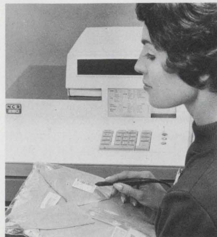
Hand-held "light wand" on fiber optic cable reads color-bar codes on articles bought in retail stores, automating and recording the sale.
