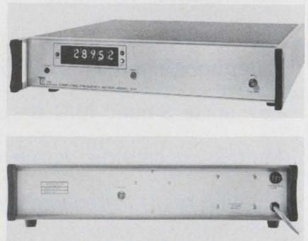
Front and rear panels of 1-MHz computing counter do away with control knobs for fully automatic operation.
