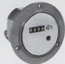
**Model T5BB**—Economical use-time indicator. Scale to 9999.9 hours, with tenths in red. Non-reset. 110 V., 60 hz. Panel mount. 2.88" dia.
