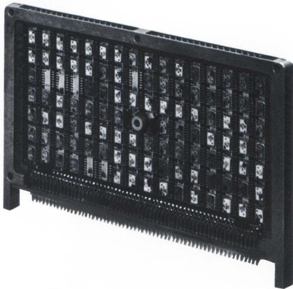
The second SUHL equipped Arma computer is an 18-bit word, parallel-organized system that weighs in at 9 pounds and takes up 0.2 cubic foot of space. This is the computer selected for use in the area navigation system of the new Lockheed L-1011 TriStar passenger jet. This computer uses 495 SUHL circuits of 9 different types, including a number of functional arrays. Again, Arma selected SUHL TTL circuits for their high noise immunity, fan-in/fan-out capability and high reliability.
