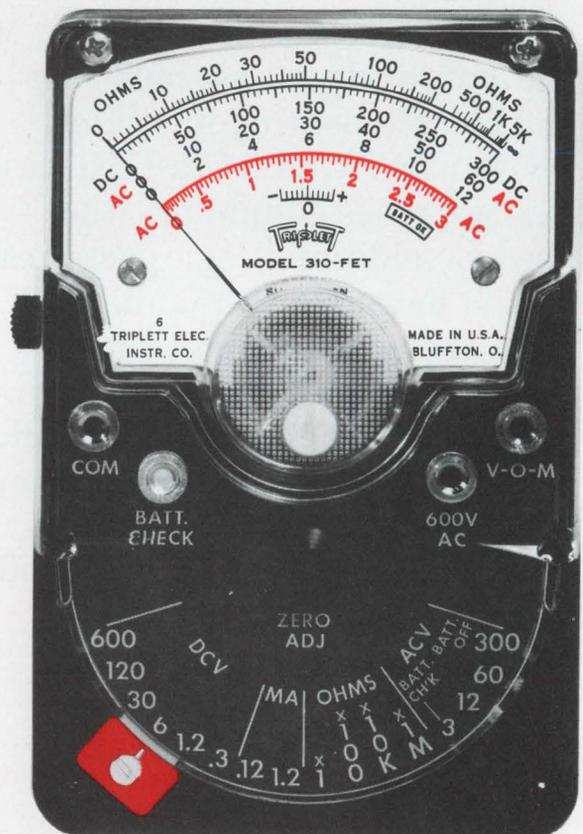
1. All Solid-State (F.E.T.) with 10 Megohm input resistance, battery operated.
