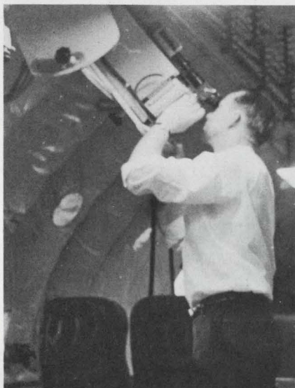
One of the two laser-referenced interferometer spectrometers is aimed by engineer Robert Pierce. Instruments are sensitive in 1- to 8-micron band and have nitrogen-cooled detectors.
