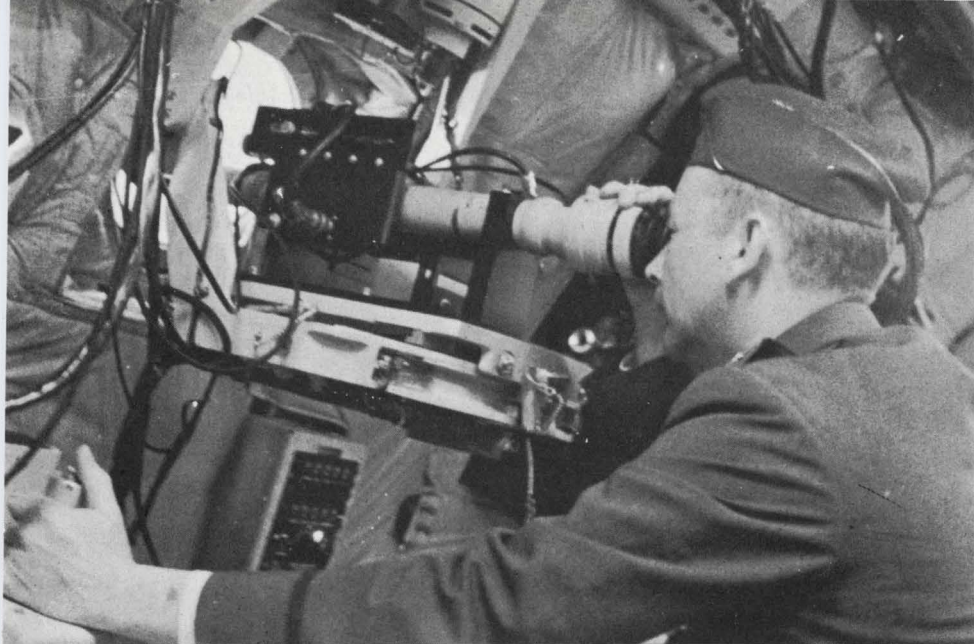
The servo-controlled master tracking station is positioned by Maj. William Grieder with a joystick control. Located on the mount is a 16-mm gun-sight camera, a narrow-band photometer and a wide-field telescope for aiming and tracking. Two other mounts are slaved to track with this station, permitting as many as seven instruments to be aimed simultaneously.
