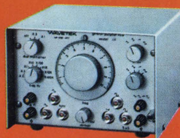
Wavetek Model 111 VCG generates sine, square, triangle, and ramp waves from 0.0015 Hz to 1 MHz, and offers precision control of the frequency of the waveforms by external voltage.
