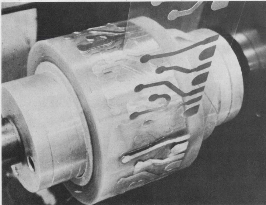
Typical dies (upper left) are for insulation material and copper foil, respectively. The die-cut circuit with Mylar release backing is shown feeding onto rewind reel. By application of insulating material, circuit is finished (upper right).
