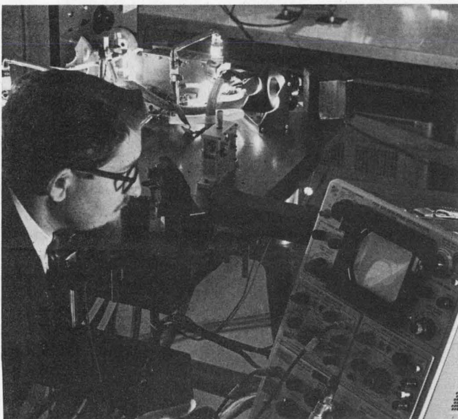
Dual laser system for phase control is shown in this block diagram (right). The key was the development of a gas laser operating right near the frequency of the 1.0582 pulse laser. Irving Itzkan checks output on scope (left).
