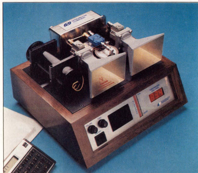
A coplanar delay that superconducts at 77°K is the key component in the FMCW radar unit from Superconductor Technologies.
