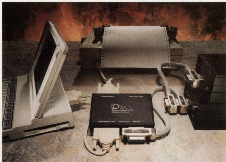
The 5.5" x 4" Personal488/NB enables 170 Kbyte/s IEEE control of up to 14 instruments
