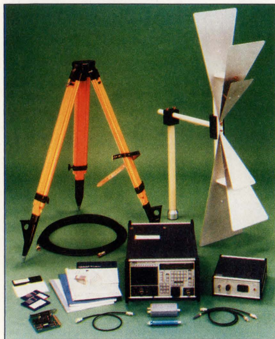
The Easy 1 turnkey emissions-assessment system from Farnell enables you to make conducted-, and radiated-emissions measurements for EMC precompliance. The kit includes one broadband antenna for covering 30 MHz to 1 GHz, LISN, an IEEE-488 PC interface card, and Easy 1 and Windows 3 software.
