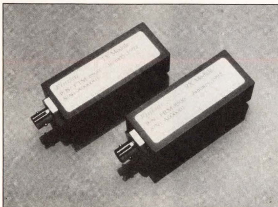
These fiber-optic transmitter and receiver modules use low-cost multimode optical components to send data at 1.5 Gbps over fibers as long as 500m.
