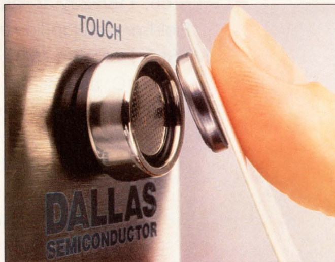
Coin-shaped data carriers from Dallas Semiconductor use only two electrical contacts to transfer data to and from their battery-backed SRAM. In the application shown here, an adhesive-backed data carrier is attached to an employee badge. Each carrier contains a readable, but unalterable, serial number that provides identification for access control.
