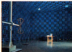
Anechoic chamber (FCC Filing and 10m Regulations)
