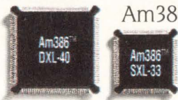
The 40MHz DXL-40 and the 33MHz SXL-33 are available in low-cost POFP packaging.
