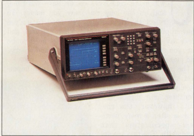
A 2-GHz bandwidth for less than $20,000 is available in the digital sequential sampling PM3340 from Philips.
