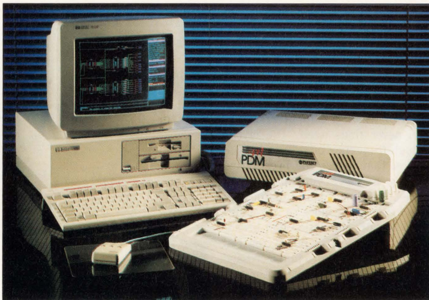
You can work in both the analog and digital realms using GEC Plessey Semiconductors' PDM prototype modeling design kit. The system lets you design, capture, simulate both digital and analog, and emulate a complete mixed-signal ASIC before committing it to silicon.
