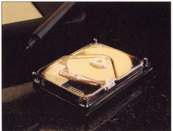
Weighing in at only 3.35 oz, the Mustang 1820 disk drive from Integral Peripherals stores 20 Mbytes in a 1.8-in. form factor.
