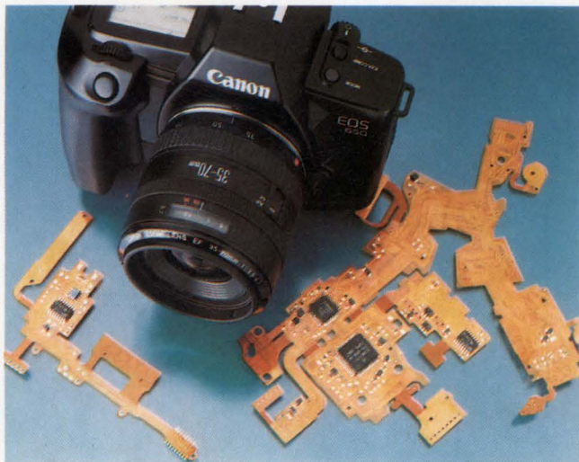
A natural application for smart-power ICs, this 35-mm autofocus camera from Canon uses two Motorola MPC1710A motor-control circuits—one to rewind the shutter spring, and one to advance and rewind the film. All circuits in the camera are under the control of Motorola's MC68HC11 microprocessor.
