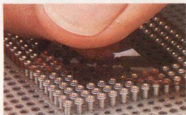
After the VIP socket is wave soldered into place, the carrier is removed to permit visual inspection of the terminals.
