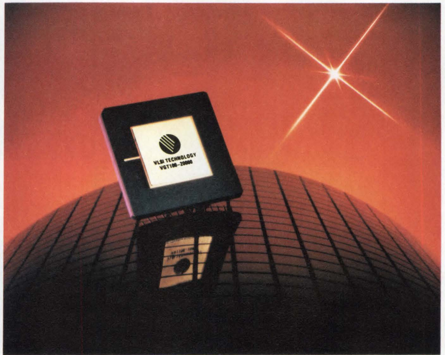
Pin-grid arrays provide more leads than any other package. VLSI Technology offers 84- to 149-pin packages in its plastic PGA product line; the company's ceramic PGAs are available in 68- to 224-pin versions.
