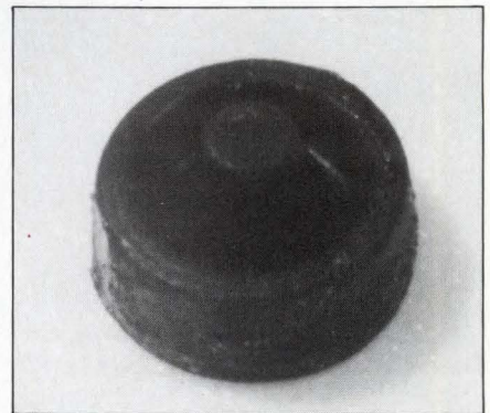
Fig 1—This all-conducting switch from Digitran measures about \frac{3}{16} of an inch in diameter. The switch fits nose down over the center contact just visible in the lower left-hand corner; a switch plate and keycap hold it in place. The switch's long nose keeps the outer wall of the switch from touching the contact encircling the center contact unless you depress the switch.
