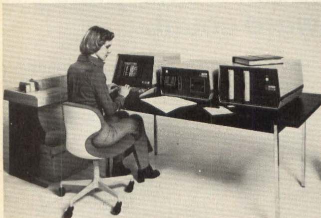
Fig 1 Tektronix 8002 microprocessor development system presently supports 8080, 6800, Z-80, 9900 and 8085 microprocessors, with other microprocessors to be added in future.
