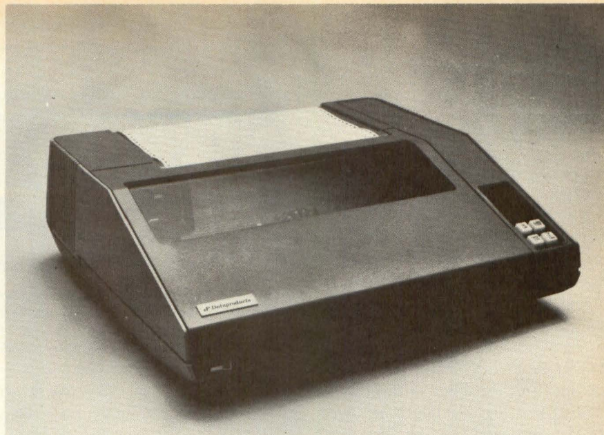
Fig 2 One of several new Dataproducts' printer entries during 1977 was the M-200 impact serial matrix printer, with a 14-element head and speed of 200 lpm
