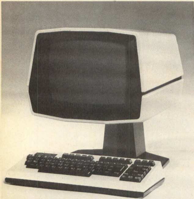
Fig 2 TEC's Model 70 microprocessor-based video display terminal uses Intel 8080 firmware to direct all video control logic and I/O functions.
