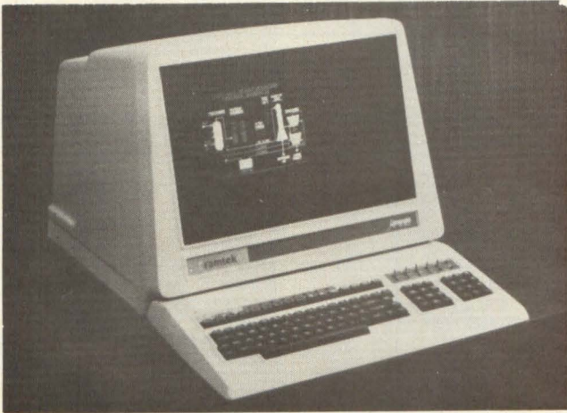
Fig 3 Ramtek's 6000 series Micrographic terminal displays graphics and alphanumeric in color or black and white.
