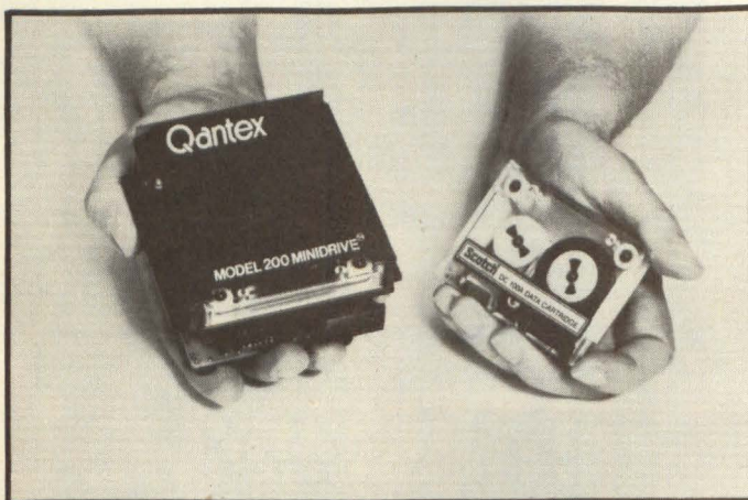
Fig 1 The Qantex Minidrive uses a minicartridge developed by 3M that contains 140 feet of 0.150-inch tape in a package measuring 2.4 x 3.2 x 0.5 inches. The transport employs a servo loop that includes a solid state optical tachometer for precise speed control of the low inertia DC motor.
