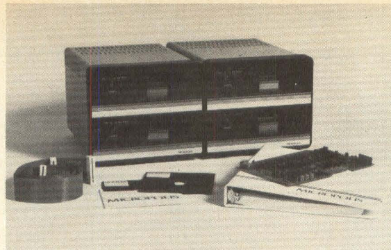
The 5.25" floppy disk in this Micropolis 1054 Mod II System stores 1.26 megabytes.
