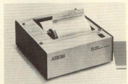
Fig 4 Axiom EX-800 electrostatic printer prints 80 columns of data on 5" paper at 160 cps.
