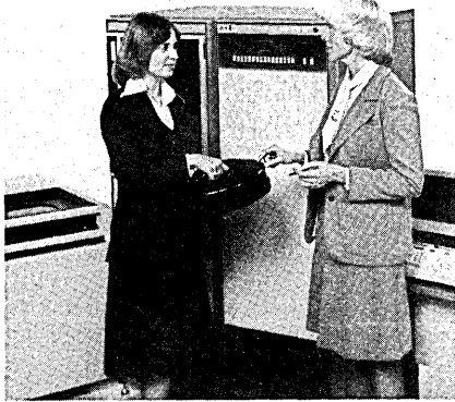
THE H-P 3000 SERIES III New processor features use of 16K semiconductor memory chips
