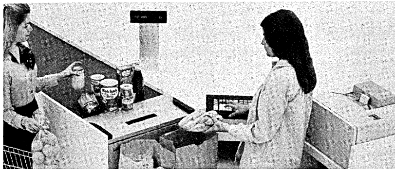
ONE EASY MOTION: IBM's new supermarket system makes it possible for a checker to check and bag in one motion. Items are simply pulled over the scanner embedded in the slot, then bagged.
