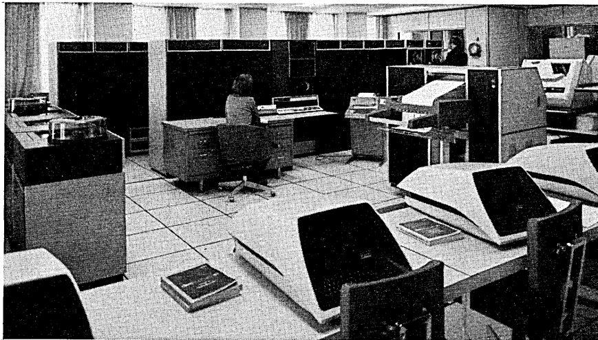
Fig. 2. Central control consists of a DECsystem-10, PDP-8/I and peripheral units.
