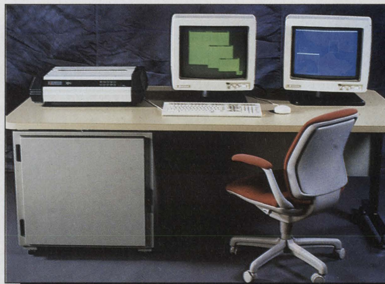
Star Technologies' processor interfaces with the VAXSTATION II/GPX over a DR11-W.
