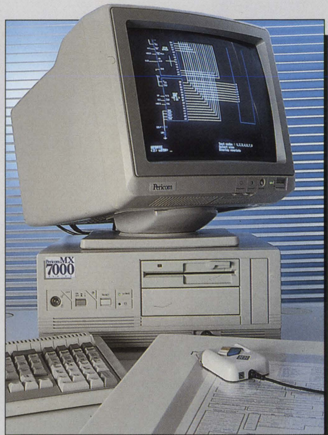
Pericom MX7000 Series workstations can function as DEC- and Tek-compatible graphics terminals or can operate in standalone mode.
