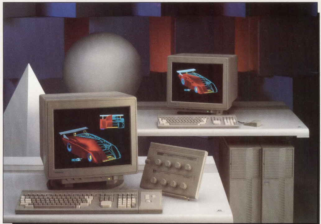
The 4337 (foreground), shaded surface 3-D system, and the 4335, a 3-D graphics workstation, combine industry computing standards with parallel graphics and compute processors.
