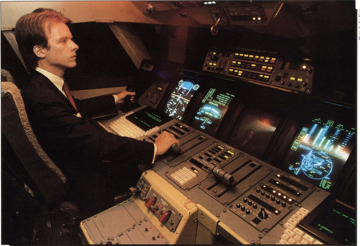
The Advanced Concepts night flying cockpit simulation. The red illumination helps pilots maintain their night vision.
