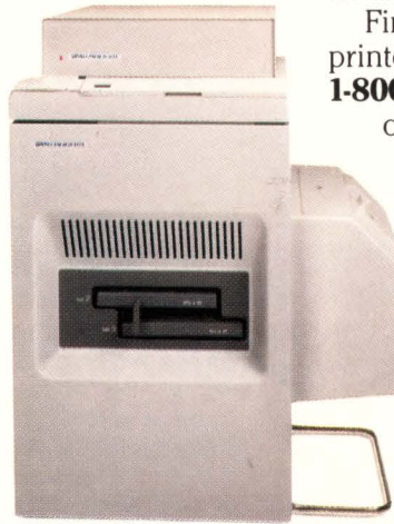
QMS Lasergrafix 2400 24-page-per-minute output up to 11" x 17" in size
