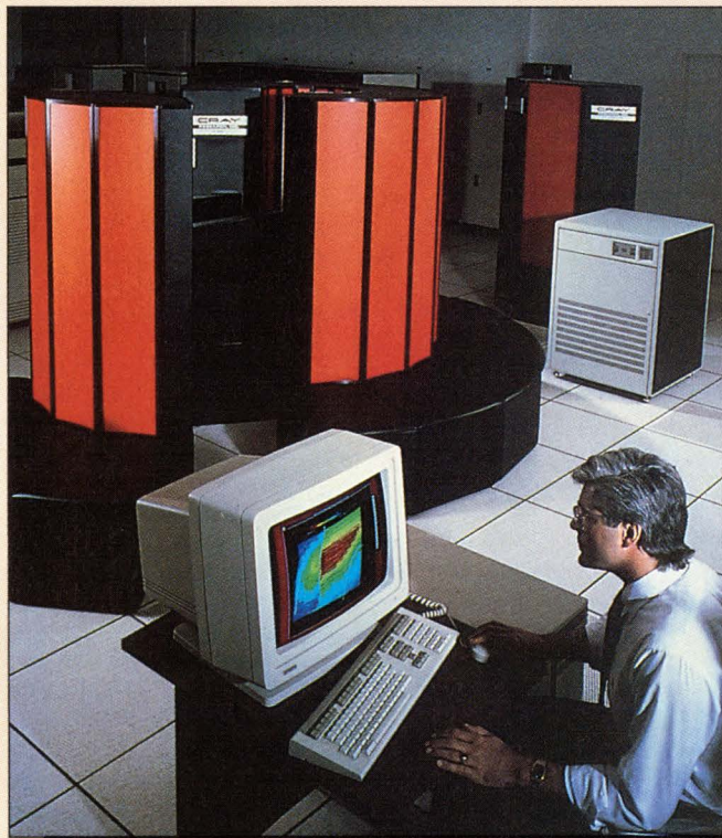
Reservoir simulation, which is a technique used for determining oil and gas reserves, is shown on a VAXstation II/GPX workstation.
