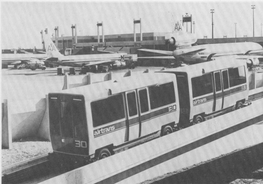
Figure 3: The Dallas-Ft. Worth airport has the largest people mover system, covering 12.5 miles of guideway.
