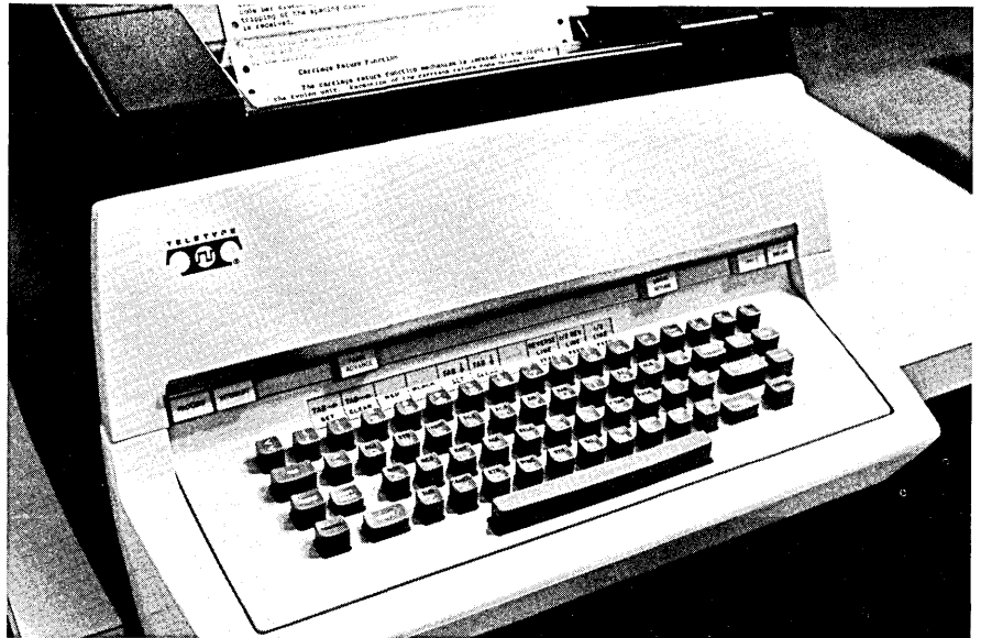
MODEL 37 KSR (KEYBOARD SEND-RECEIVE) SET / Teletype Corp., Skokie, Ill. — The ability to operate at 150 words per minute (15 characters per second) and print 128 graphics are key features of the Model 37 KSR Set. First in a full line of data communications equipment, it is designed to use the complete U.S.A. Standard Code for Information Interchange (USASCII). It also can be used as a computer input/output device and has applications in such office routine as the preparation of sales orders and other business forms. (Circle #96 on the Reader Service Card.)
