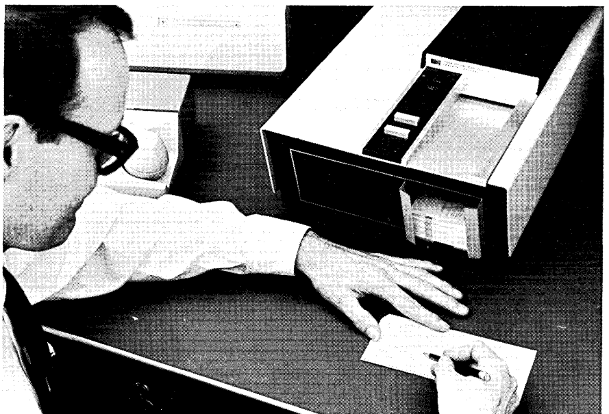
MODEL 2760A OPTICAL MARK READER / Hewlett Packard, Palo Alto, Calif. — Tab cards to be read by the Model 2760A may be all punched, or all marked in soft pencil, or any combination of the two. Errors in pencilled entries can be erased. Reading rate and output format of the reader are compatible with standard telephone data sets, and appropriate for simple data communication situations using Teletype, Data-Speed, or other tape perforators. Standard rate is 105 characters per second; 10 characters per second is optional. Model 2760A is available both to OEM and user markets. (Circle #97 on the Reader Service Card.)
