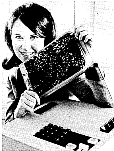
— Karen O'Donnell, IBM, holds 1000 inches of magnetic recording tape snaked in a specially-designed plastic cassette
