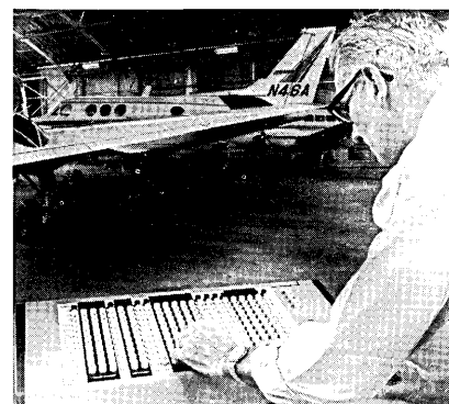
— C-Dek® data entry keyboard being used to record aircraft maintenance accounting information.
