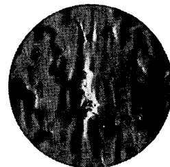
OTHER POLYESTER FILMS. SURFACE MAGNIFIED 400X. (UNRETOUCHED PHOTO-MICROGRAPH.)
