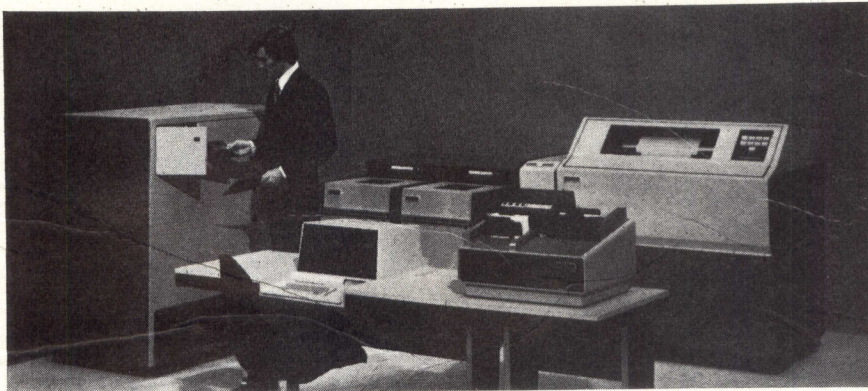
Occupying only 10 sq ft of floor space, NCR's Criterion 8550 mainframe (left) combines MSI and LSI circuits with up to 1M bytes of MOS memory in the same cabinet. The processor's internal transfer bus uses distributed-intelligence techniques to eliminate processing bottlenecks; flexible firmware provides multiple-virtual machine capabilities
