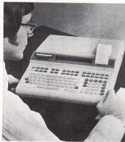
Live keyboard on Hewlett-Packard's 9825A desktop programmable calculator permits calculations to be made at the same time that the calculator is running control programs. At top front of unit, from left to right, are tape drive (for minicartridges), 32-character LED display, and 190-line/min. thermal printer
