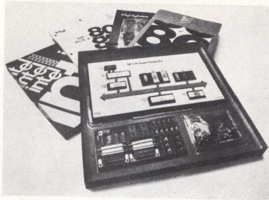
Intel Corp's MCS-80 micro-computer system design kit. All necessary components are included to build a complete 8080A-based system. The board also provides area for system expansion and for custom interfacing
