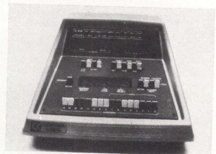
Programmer's console for MM1 micro-computer. The desktop unit plugs into the computer's "Poly-Buss." Controls include reset, run, halt, cycle step, instruction step, and interrupt enable/disable
