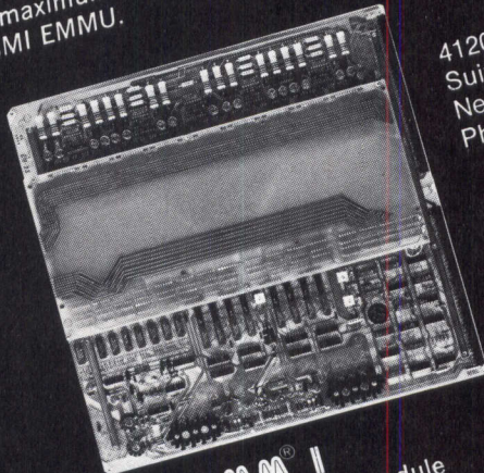
PINCOMM® A16K 16,384 words on a single PCB for the GA SPC-16.
