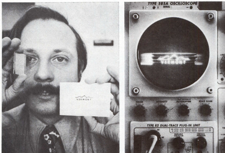
Fig. 10 Results. Author displays sketch that was illuminated and focused on a section of the 1- x 1.6-in. area scanner chip (left). The chip produced the picture on the oscilloscope (right)
