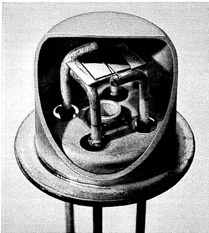
Fig. 6 — Construction of the radiation damage transistors.
