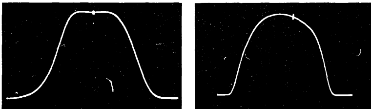
(b) GAIN-FREQUENCY CHARACTERISTIC OF IF AMPLIFIER USING COUPLED-RESONATOR REFLEX KLYSTRON AS SWEEP SOURCE CENTER FREQUENCY OF IF-AMPL = 70MC FLAT BANDWIDTH OF IF-AMPL = 22 MC
