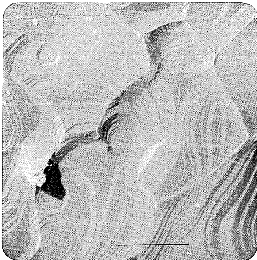
Fig. 14—Germanium replica ( i_e \approx 150\text{\AA} , \theta_a = 35^\circ ) of near optimum thickness. Resolution about 75\text{\AA} . Ruptured film evident in shadow.
