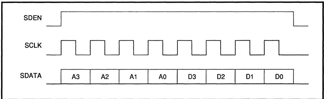
**FIGURE 2: Serial Port Timing**
