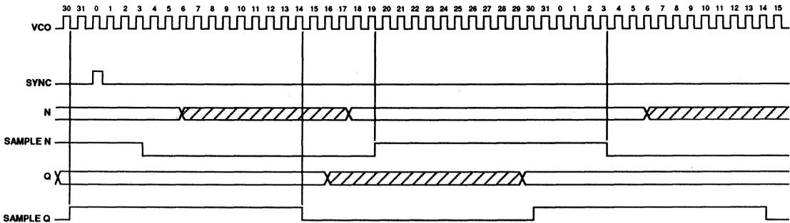
FIGURE 2: Dedicated Servo Timing Diagram
