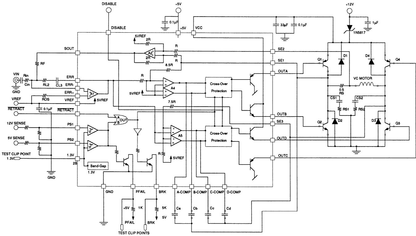
FIGURE 2: SSI 32H6240 Typical Application
