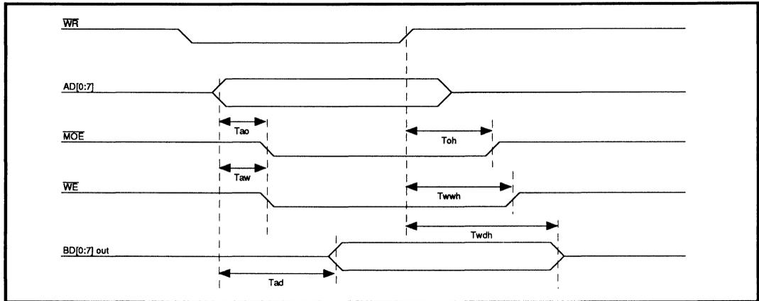
**FIGURE 8: Register 70H Write Timing**
