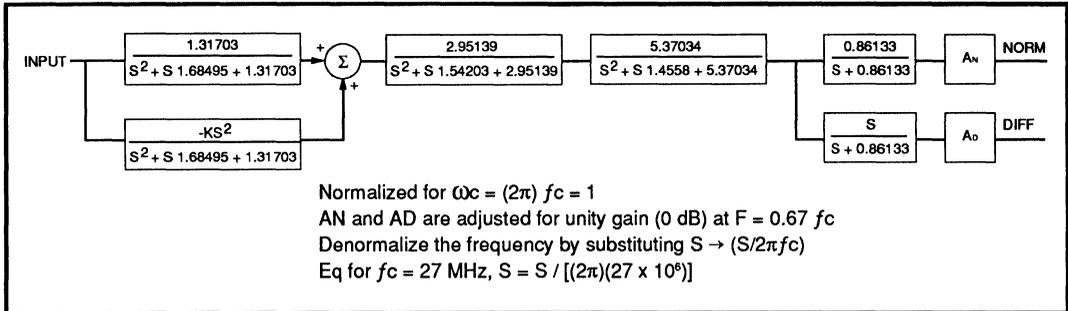
**FIGURE 5: 32F8000 Normalized Block Diagram**
