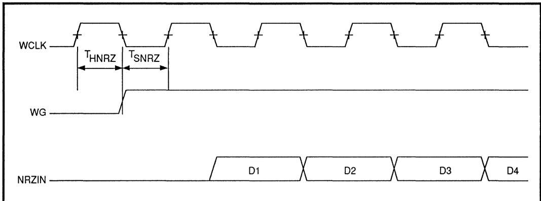
FIGURE 5: WG Timing Requirement for Predictable Write Encoding
