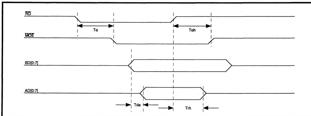
**FIGURE 10: Register 70H Read Timing**
