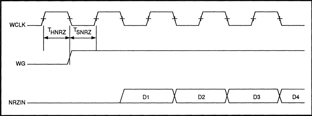
**FIGURE 3: WG Timing Requirement for Predictable Write Encoding**
