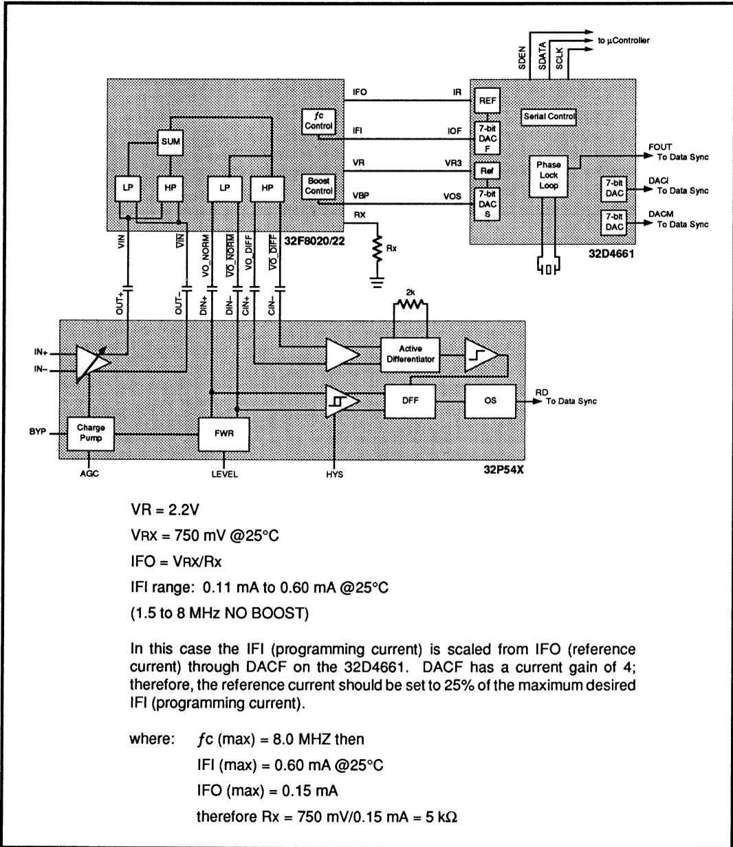
**FIGURE 2: Applications Setup, Constant Density Recording
