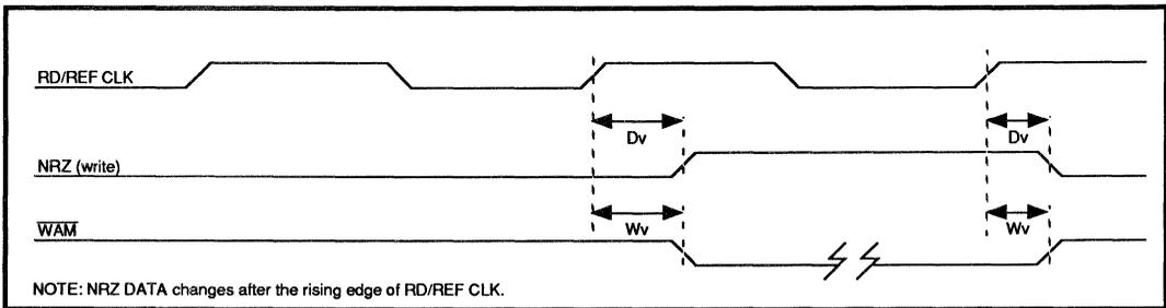
FIGURE 6: Disk Write Timing
