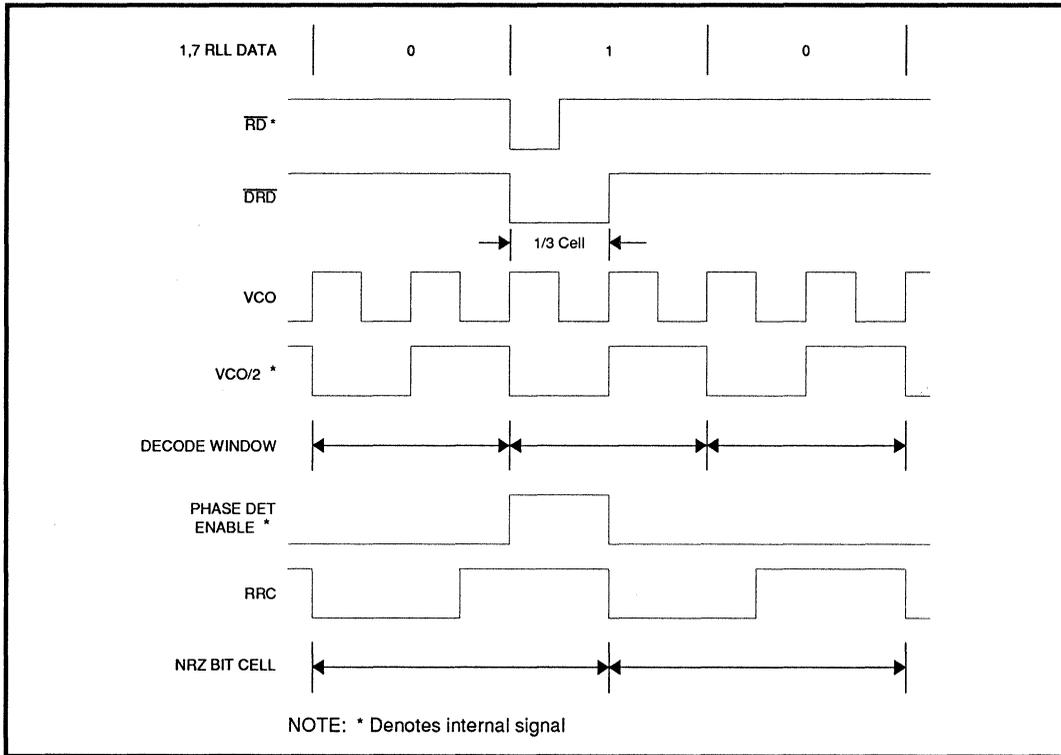
FIGURE 8: Data Synchronization Waveform
