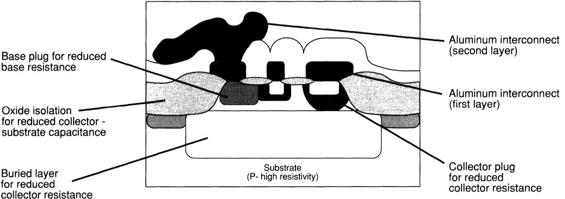
FIGURE 2: BN Bipolar Process NPN Transistor
