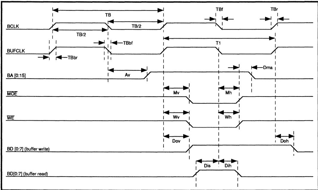
FIGURE 10: Buffer Memory Read/Write Timing
