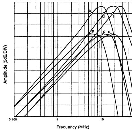
FIGURE 5: 32F8011/8012 Differentiated Low Pass Output Response (VO\_DIFF)
