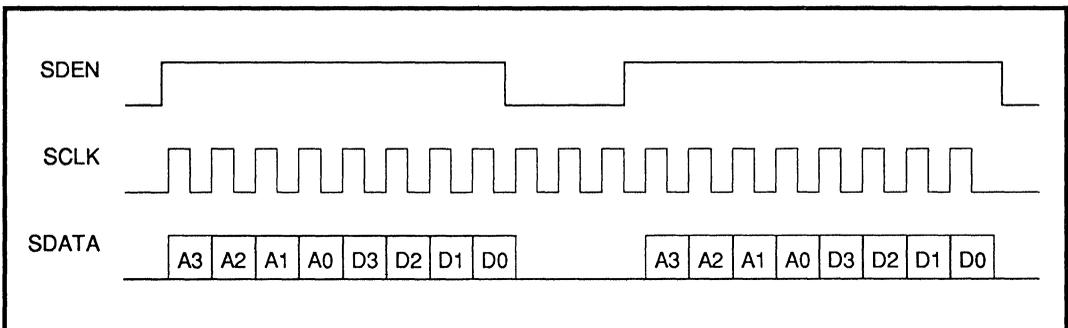
FIGURE 3: Serial Port Timing, Multiple Transfers
