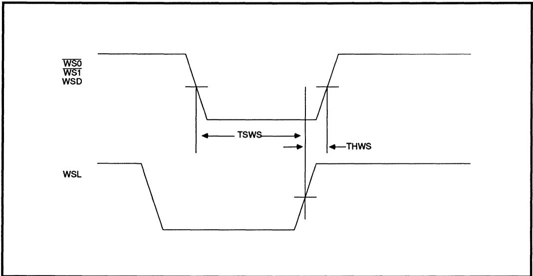
FIGURE 11: Control Timing
