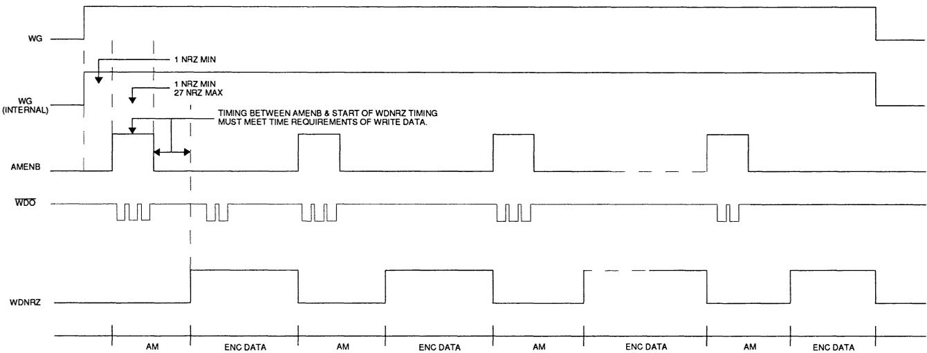
FIGURE 10: Multiple Address Mark Write
