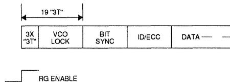
In hard sector operation  $\overline{AMD}$  remains inactive. A hard sector read operation does not require an address mark search but starts with a preamble search as with soft sector and sequences identically. In all respects, with exception to the address mark search sequence, hard sector read operation is the same as soft sector read.
