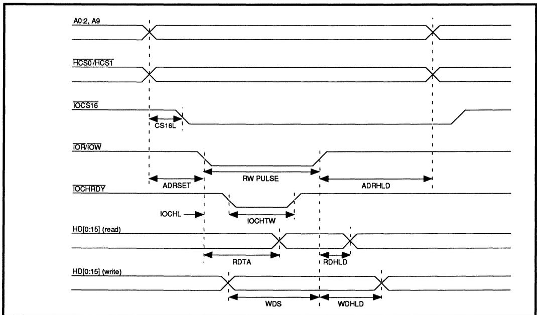
**FIGURE 3: Host Programmed 8/16-Bit Timing**
