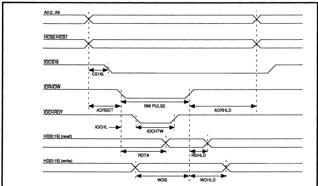
**FIGURE 4: Host Programmed 8/16-Bit Timing**
