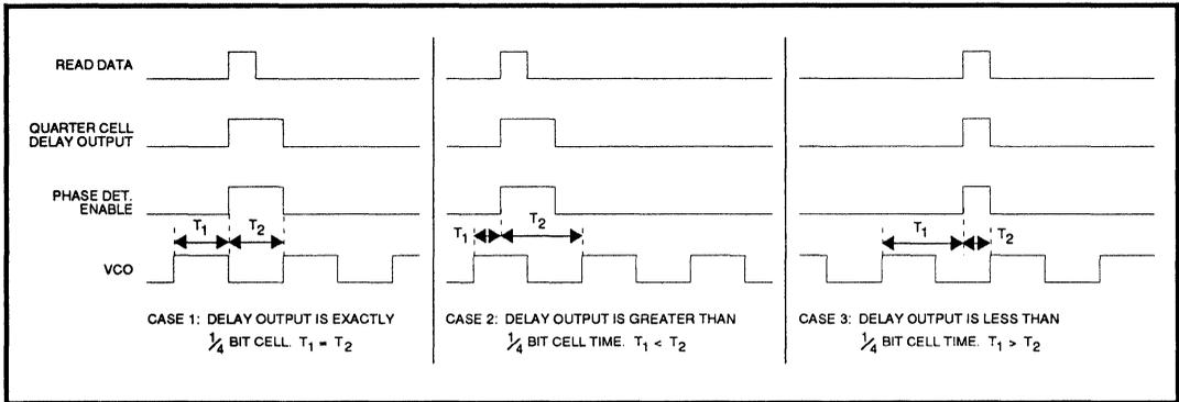
**FIGURE 18B: Timing of Phase Detector Enable Logic.** The read data input pulse can shift to the left by  $T_1$  and to the right by  $T_2$  before an error occurs in the phase detector output polarity, If the quarter cell delay output is not exactly  $\frac{1}{4}$  bit cell wide, then  $T_1 \neq T_2$ , as shown in cases 2 and 3.
