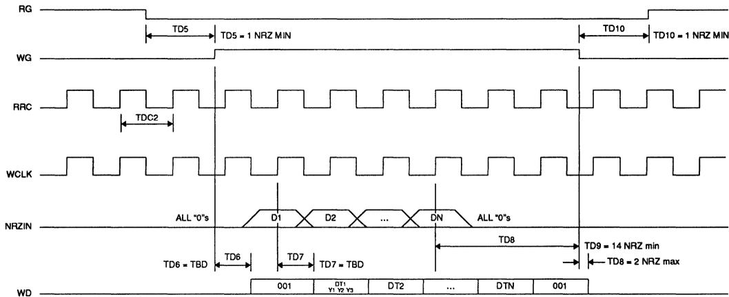
FIGURE 12: Write Mode NRZ Data Timing
