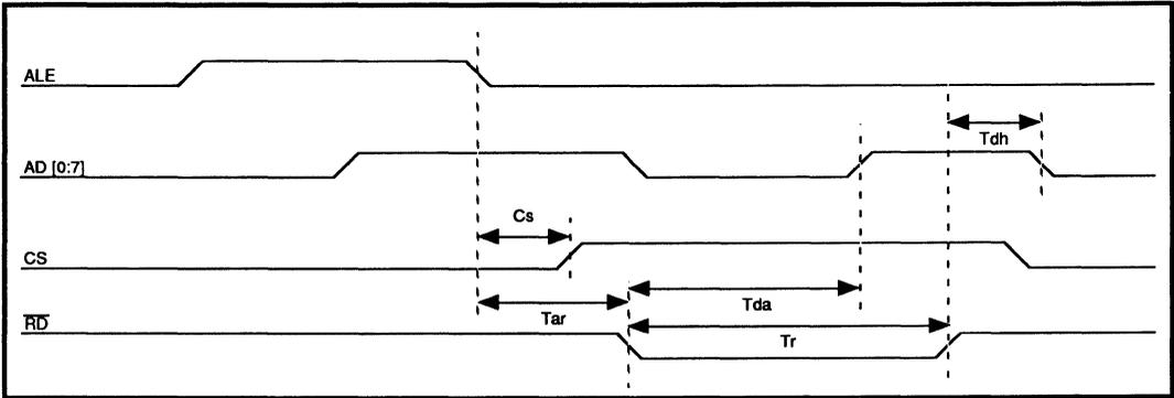
**FIGURE 6: Register Read Timing**
