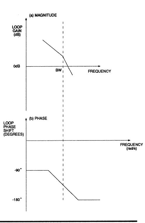
**FIGURE 12: Bode Plot of Simplified Seek Mode Transfer Function**
