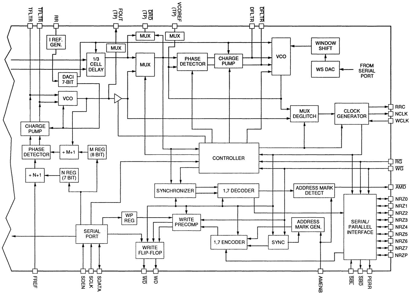
FIGURE 1(B): SSI 32P4740 Combo Device Part 2
