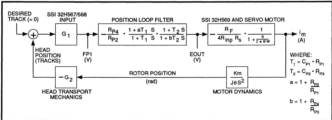
FIGURE 8(a): System Transfer Function in Track Mode
