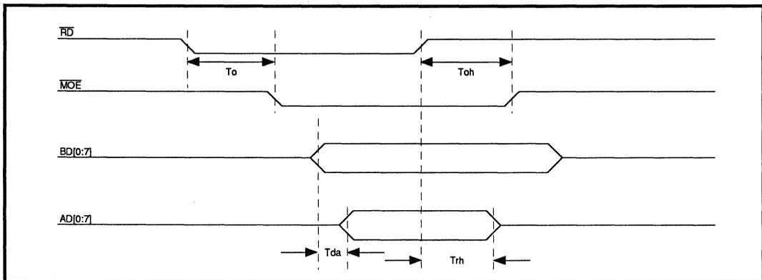
FIGURE 7: Register 70H Read Timing
