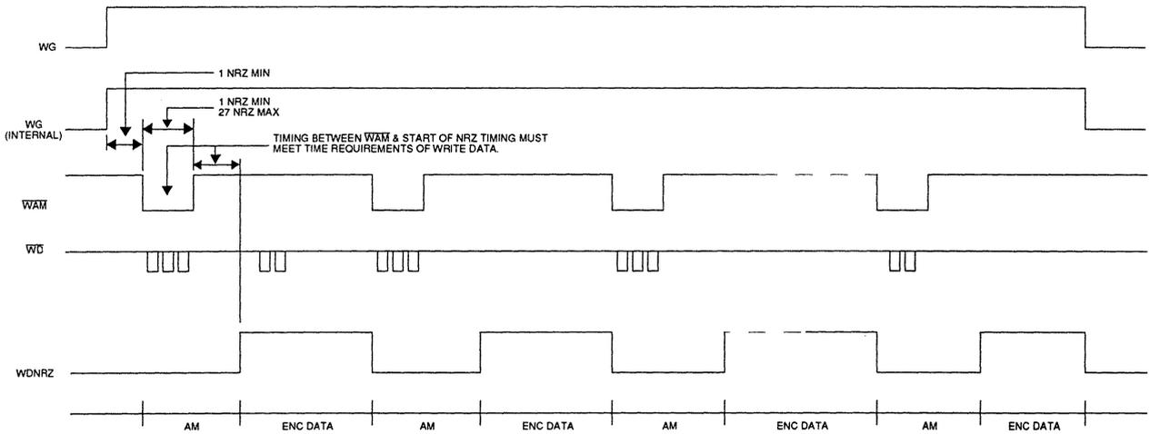
FIGURE 14: Multiple Address Mark Write
