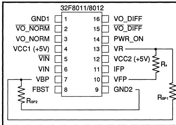
FIGURE 1: 32F8011/8012 Applications Setup, 16-Pin SO or DIP
