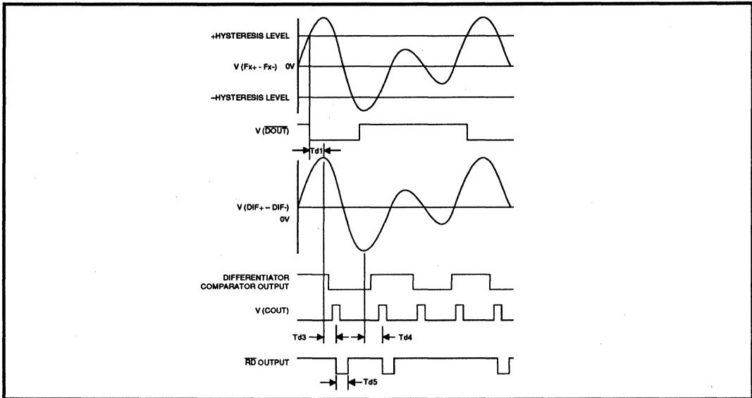
FIGURE 6: Read Mode Digital Section Timing Diagram
