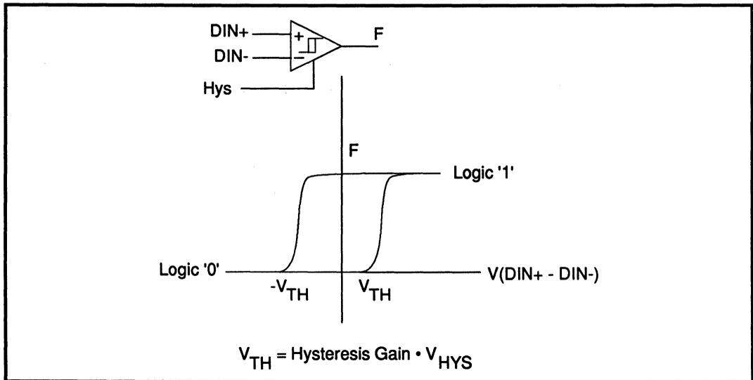
FIGURE 5b: Hysteresis Comparator Transfer Function
