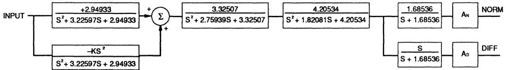
The cutoff frequency,  $f_c$ , is programmable with 3 pins: RX, IFO and IFI. At the RX pin, an external resistor to ground establishes a reference current,  $IFO = 0.75 / R_x$ , at  $T = 27^\circ\text{C}$ . IFI should be made proportional to IFO for  $f_c$  temperature stability. The cutoff frequency is related to the RX resistor, IFO and IFI currents at the following:
