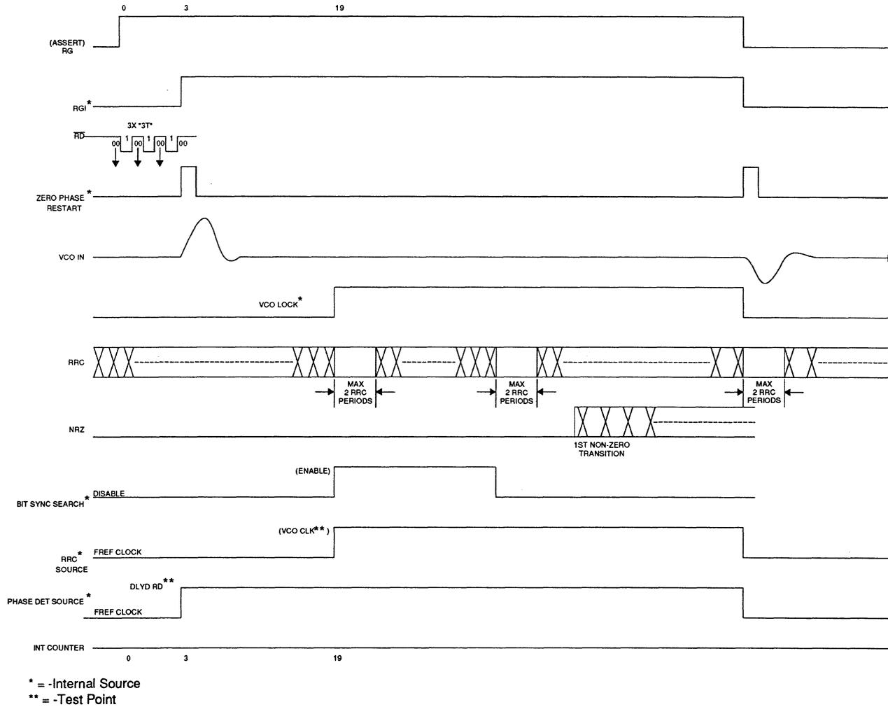
FIGURE 13: Read Mode Locking Sequence (Soft and Hard Sector)
