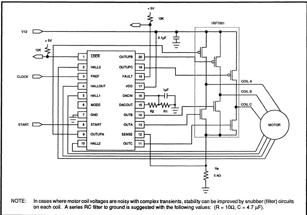
**Typical Three-Phase, 4-Pole, Bipolar,
