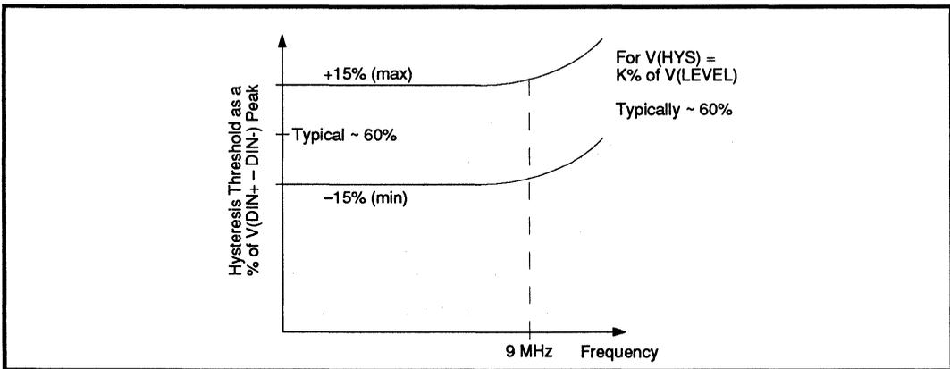
FIGURE 5: Percentage Threshold Versus Frequency
