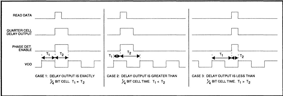
**FIGURE 18B: Timing of Phase Detector Enable Logic.** The read data input pulse can shift to the left by  $T_1$  and to the right by  $T_2$  before an error occurs in the phase detector output polarity, If the quarter cell delay output is not exactly 1/4 bit cell wide, then  $T_1 \neq T_2$ , as shown in cases 2 and 3.
