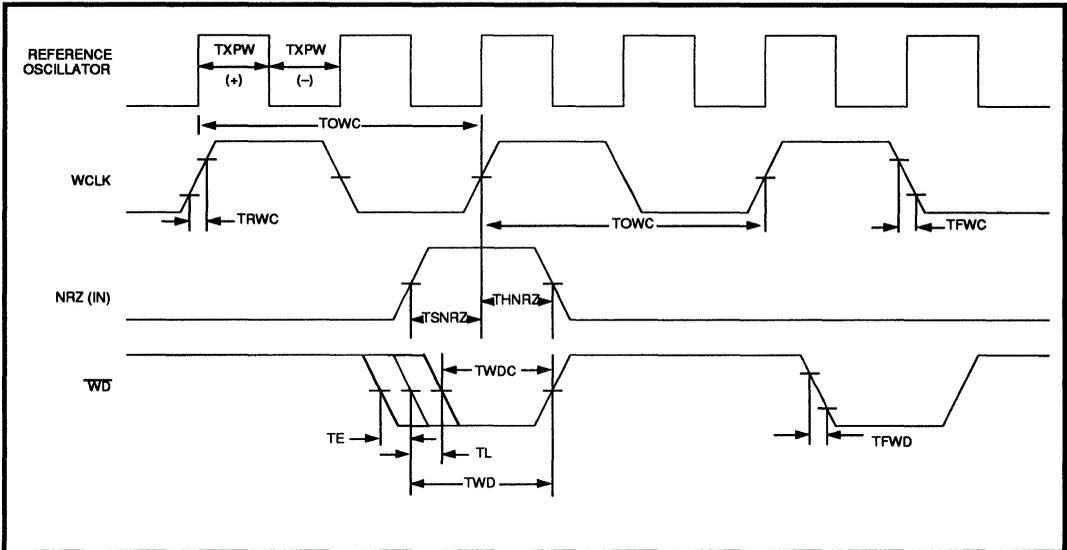
**FIGURE 10: Write Timing**
