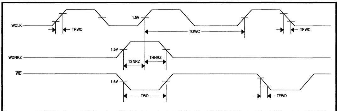
FIGURE 4: Write Timing
