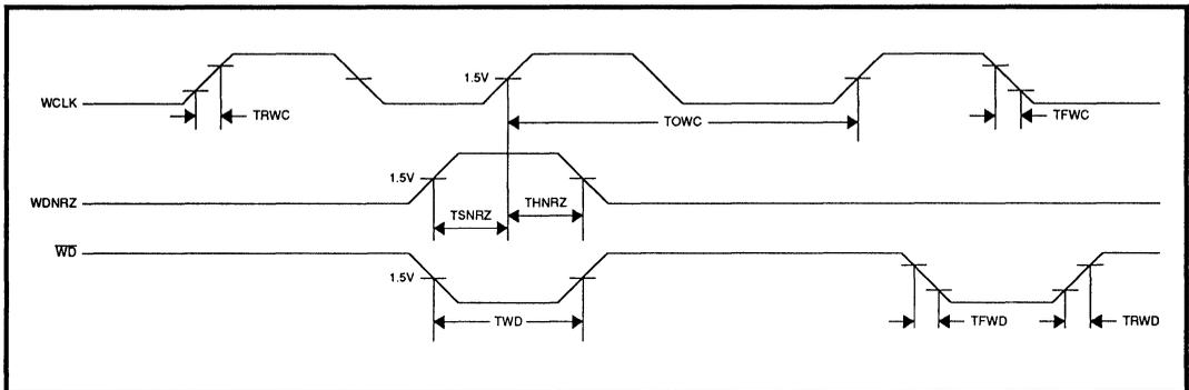
FIGURE 10: Write Timing
