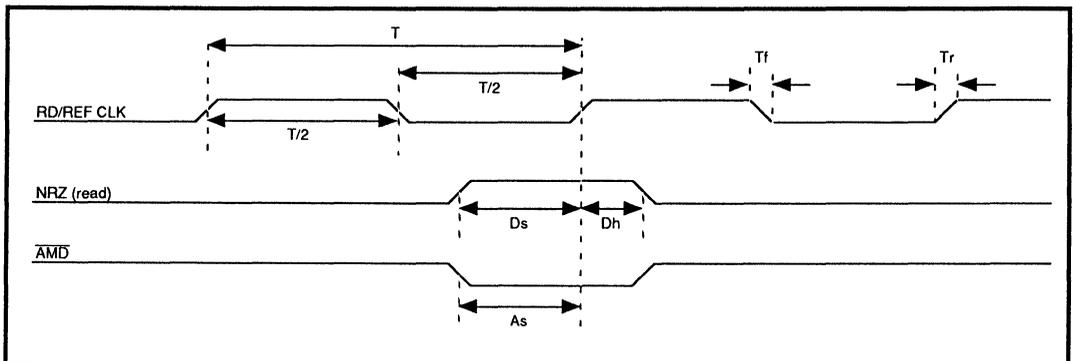
FIGURE 5: Disk Read Timing
