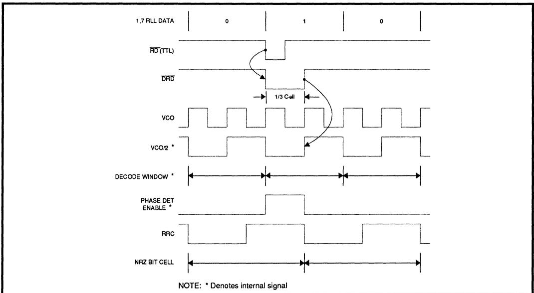
FIGURE 1: Data Synchronization Waveform
