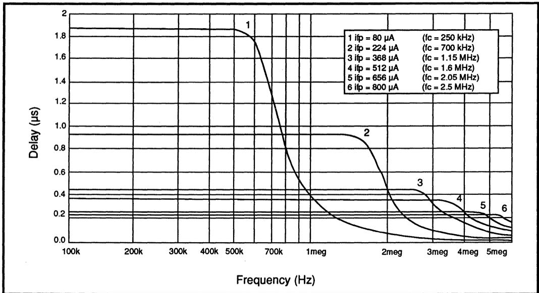
FIGURE 1: Typical Normal/Differentiated Output Group Delay Response
