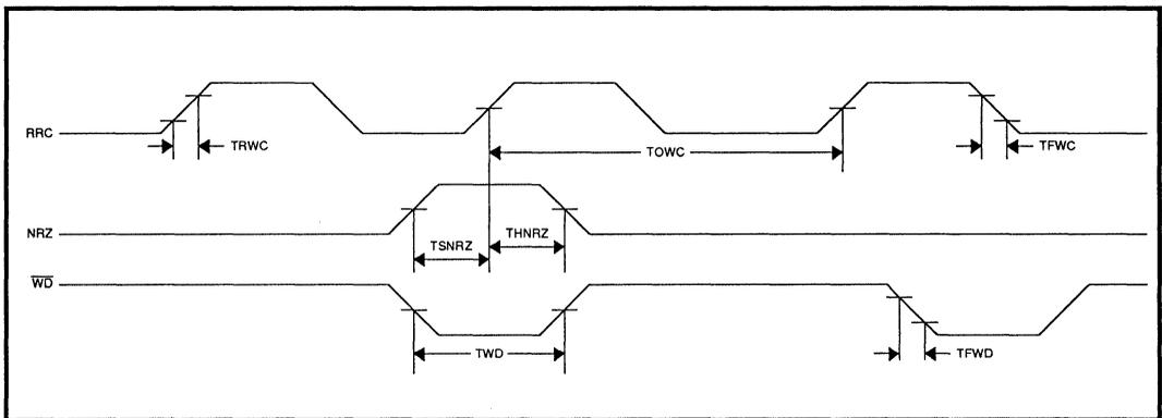
FIGURE 11: Write Timing
