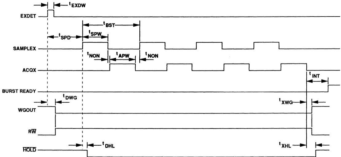
FIGURE 4: Embedded Servo Timing Diagram with External Timing Source
