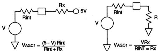
V = Voltage at AGC1 with pin open (2.2V, nom.)
