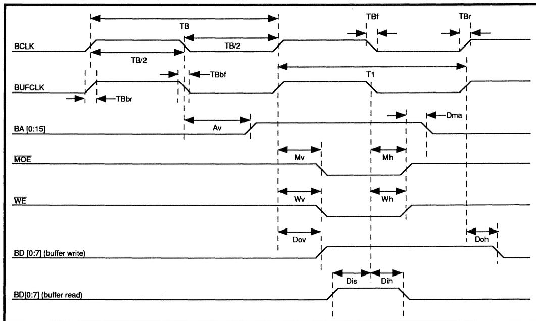
FIGURE 9: Buffer Memory Read/Write Timing
