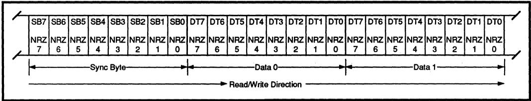
**FIGURE 14: Parallel/Serial Conversion Format**
