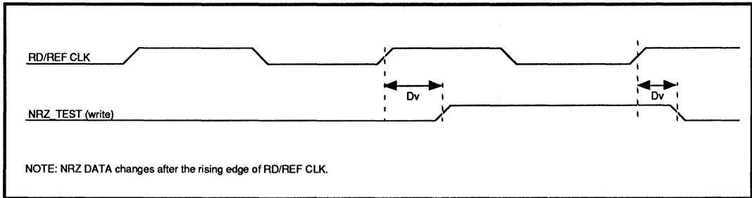
FIGURE 7: NRZ Test Output Timing
