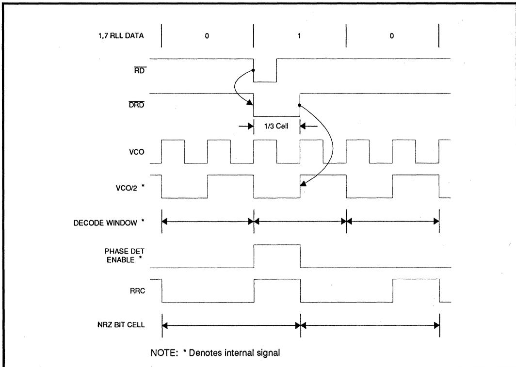
FIGURE 3: Data Synchronization Waveform
