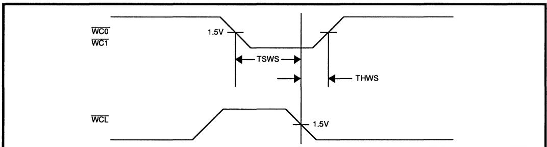
FIGURE 5: Control Timing
