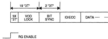
In hard sector operation a low AMENB disables the SSI 32P4720/4721's Address Mark Detection circuitry and AMD remains inactive. A hard sector read operation does not require an address mark search but starts with a preamble search as with soft sector and sequences identically. In all respects, with exception to the address mark search sequence, hard sector read operation is the same as soft sector read.
