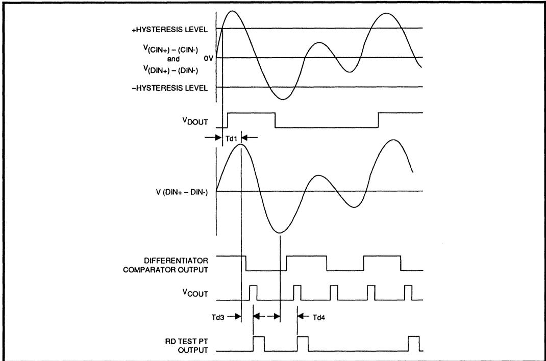
**FIGURE 8: Read Mode Digital Section Timing Diagram**
