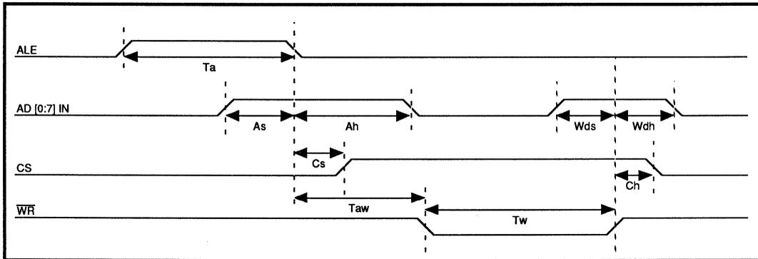
FIGURE 3: Register Write Timing
