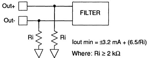
One filter for both amplitude ( $DIN_{\pm}$  input) and time ( $CIN_{\pm}$  input) channels, or a separate filter for each may be used. If two filters are used, attention must be paid to time delays so that each channel is timed properly. A multi-pole Bessel filter is typically used for its linear phase or constant group delay characteristics.
