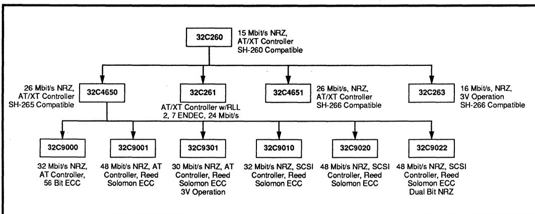
FIGURE 1: Silicon Systems' Single Chip Controller Hierarchy
