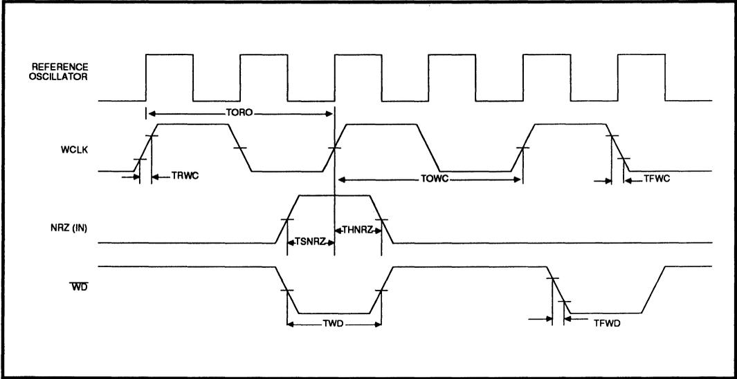
FIGURE 10: Write Timing
