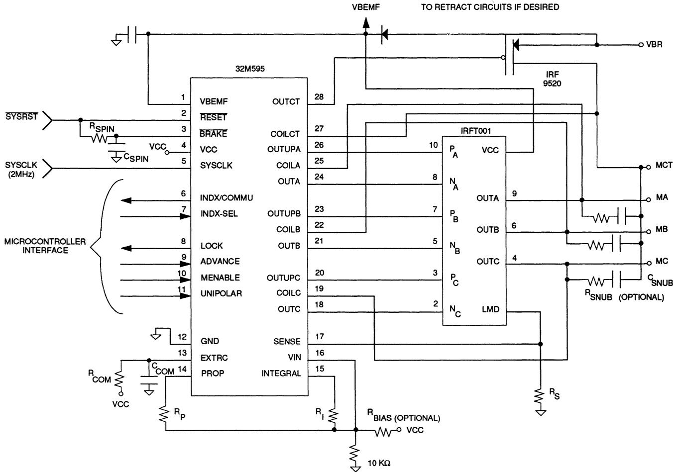
Typical Bipolar Start/Unipolar Run 32M595 Application
