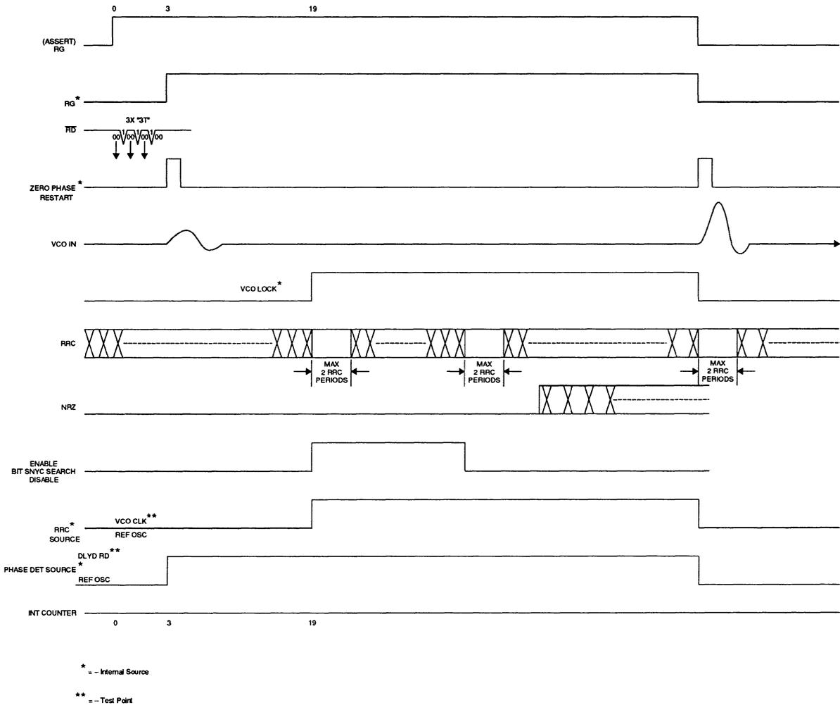
**FIGURE 7: Read Mode Locking Sequence (Soft and Hard Sector)**
