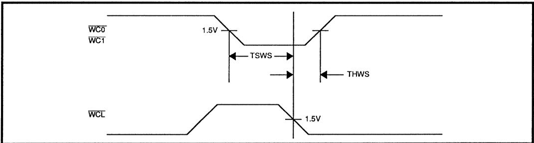
**FIGURE 5: Control Timing**
