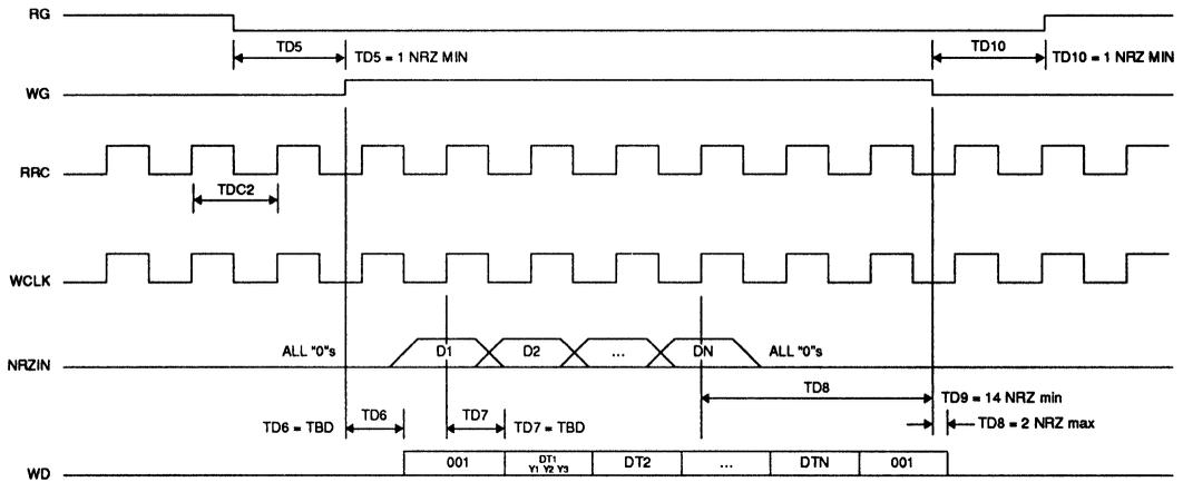
FIGURE 16: Write Mode NRZ Data Timing
