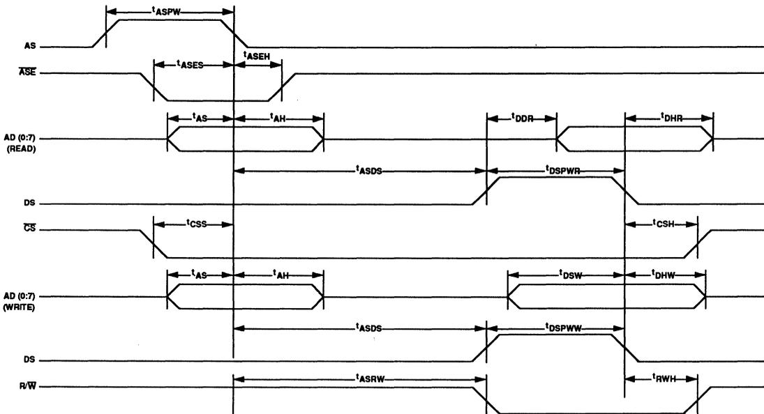
FIGURE 6: Motorola Microprocessor Bus Interface Timing Diagram
