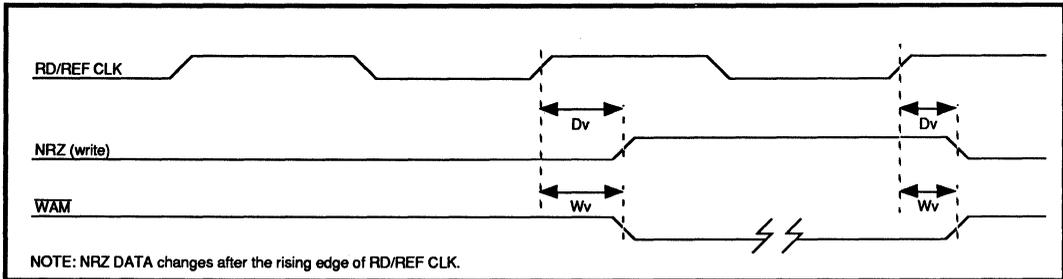
FIGURE 6: Disk Write Timing
