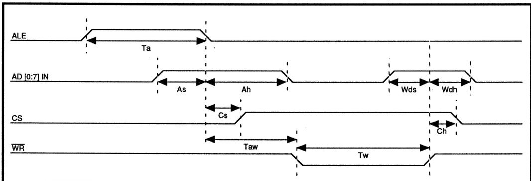
FIGURE 4: Register Write Timing
