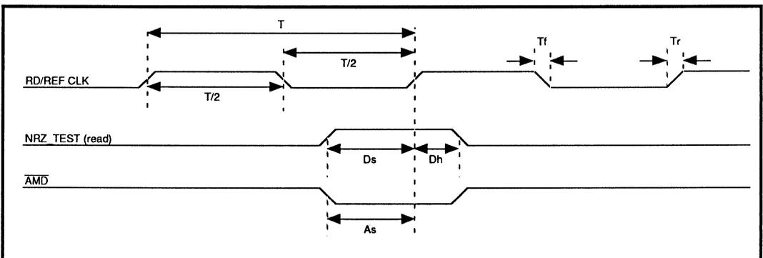
**FIGURE 6: NRZ Test Input Timing**
