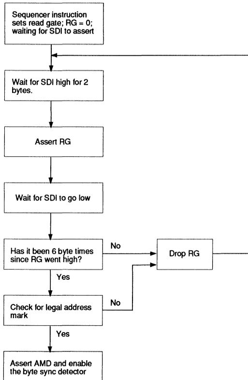
**FIGURE 1: Encoder Sequence for Soft Sector Mode**
