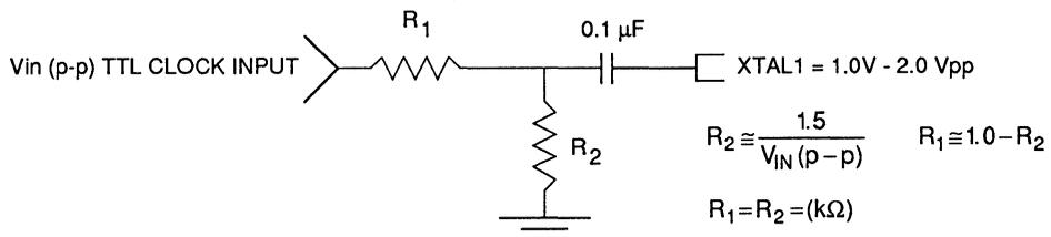
The signal amplitude into XTAL1 should be attenuated to approximately 1.0 to 2.0 V<sub>p-p</sub>; this will insure that the transients associated with TTL switching characteristics won't couple into the data synchronizer and degrade performance.
