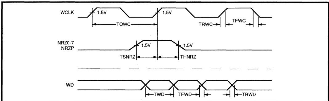
FIGURE 6: Write Timing
