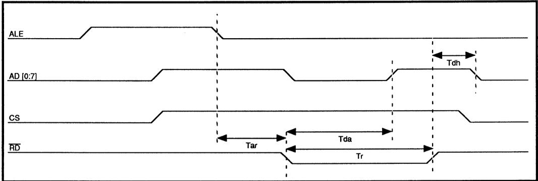
**FIGURE 5: Register Read Timing**
