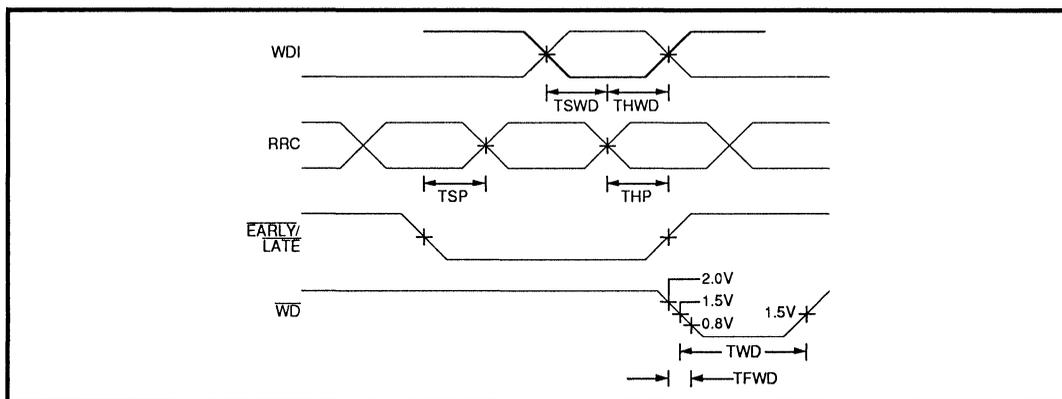
FIGURE 9: Write Mode Timing
