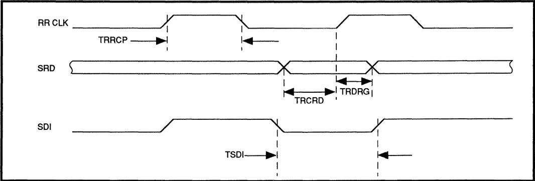
**FIGURE 12 : Read Data Timing - RLL ENDEC Mode**
