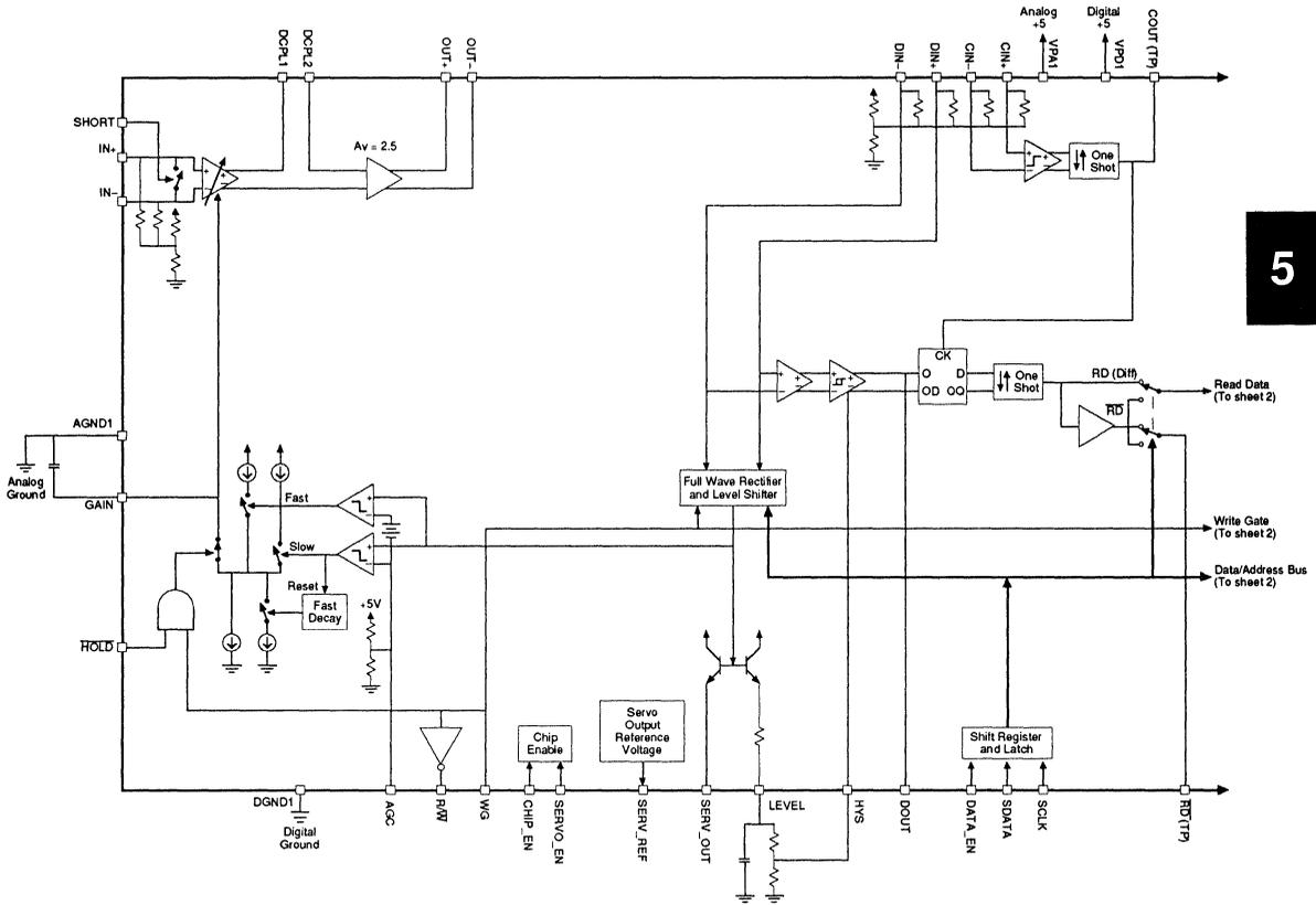
FIGURE 5a: SSI 32P4622 Circuit Block Diagram (Sheet 1)
