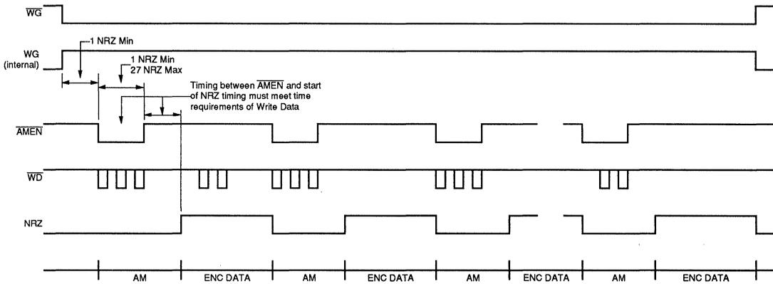
**FIGURE 11: Multiple Address Mark Write**
