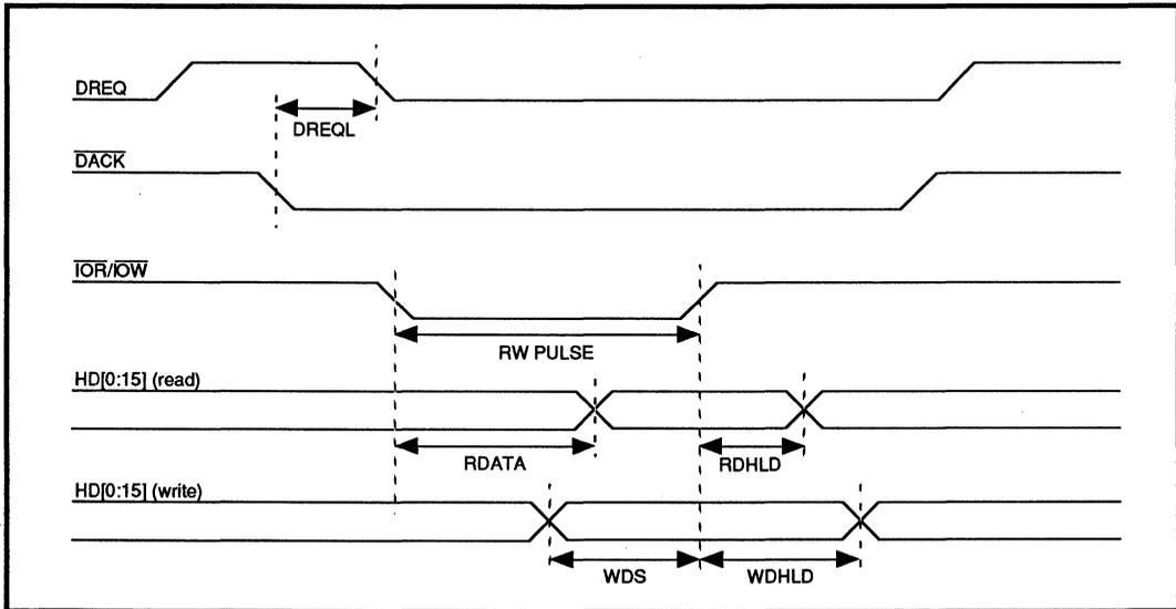
FIGURE 2: Host DMA 8/16-Bit Interface Timing
