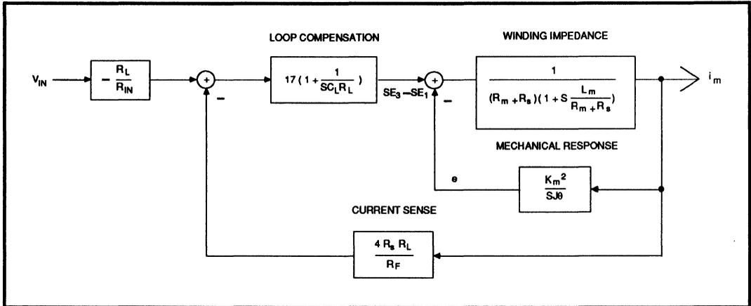
FIGURE 4(A): Transfer Function Of SSI 32H569
