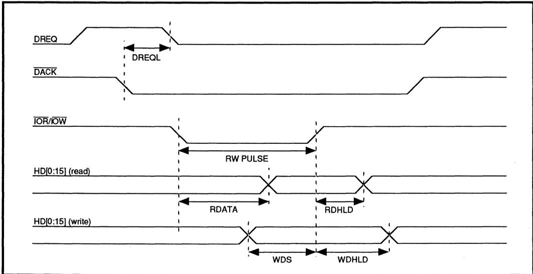
FIGURE 1: Host DMA 8/16-Bit Interface Timing
