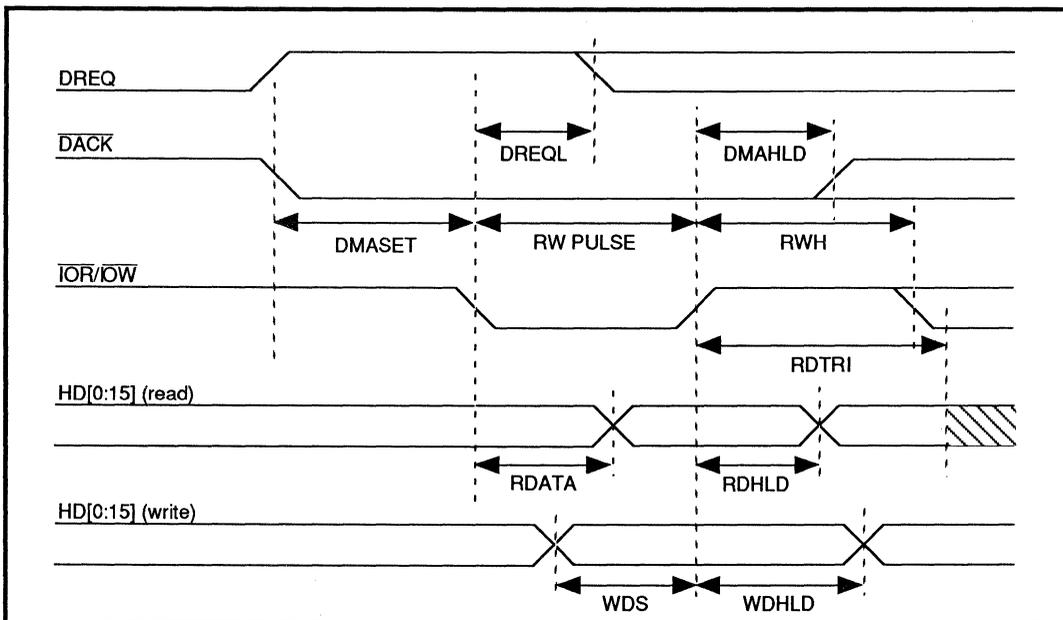
FIGURE 3: Host DMA 8/16-Bit Interface Timing (Demand Mode)
