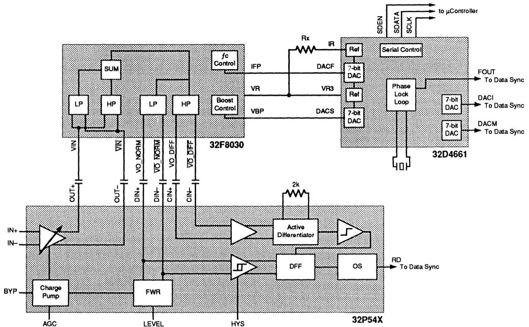
**FIGURE 2: Applications Setup, Constant Density Recording
