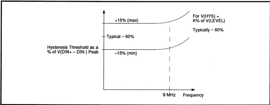
FIGURE 6: Percentage Threshold Versus Frequency
