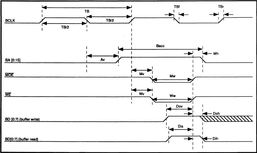
**FIGURE 12: Buffer Memory Read/Write Timing**
