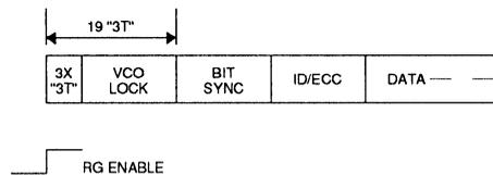
In hard sector operation a low AMENB disables the SSI 32D4010's Address Mark Detection circuitry and  $\overline{AMD}$  remains inactive. A hard sector read operation does not require an address mark search but starts with a preamble search as with soft sector and sequences identically. In all respects, with exception to the address mark search sequence, hard sector read operation is the same as soft sector read.
