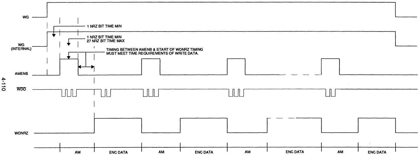
FIGURE 8: Multiple Address Mark Write
