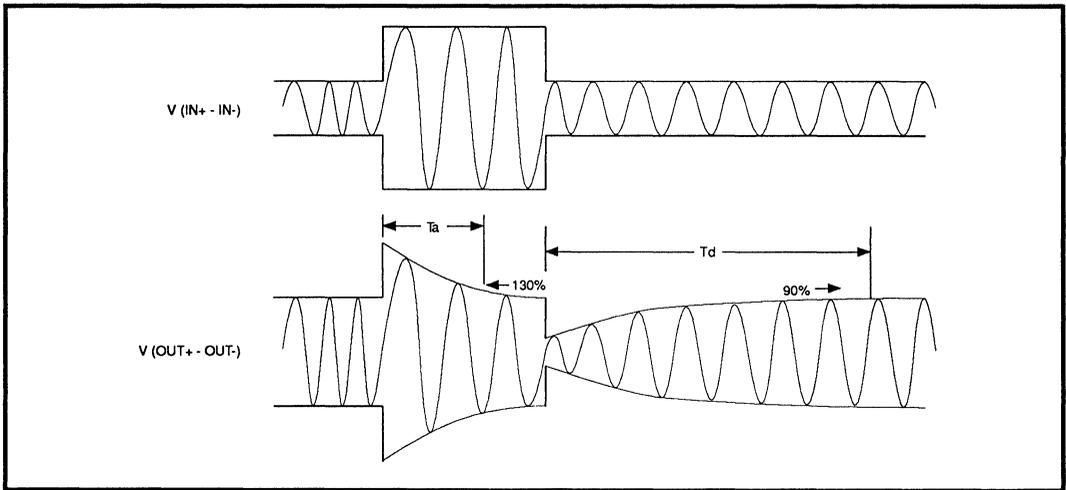
FIGURE 6: AGC Timing Diagram
