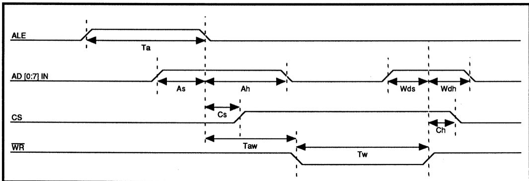
FIGURE 3: Register Write Timing
