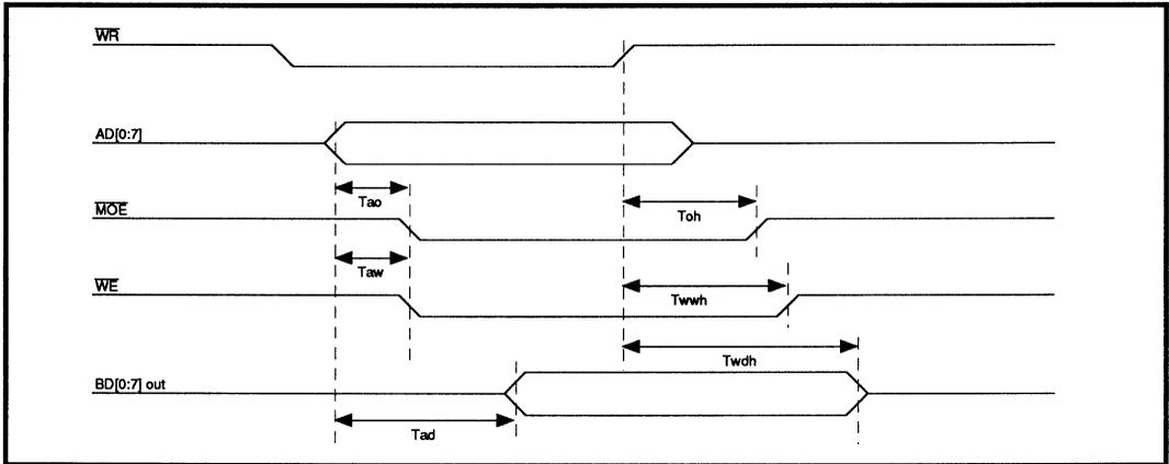
**FIGURE 8: Register 70H Write Timing**
