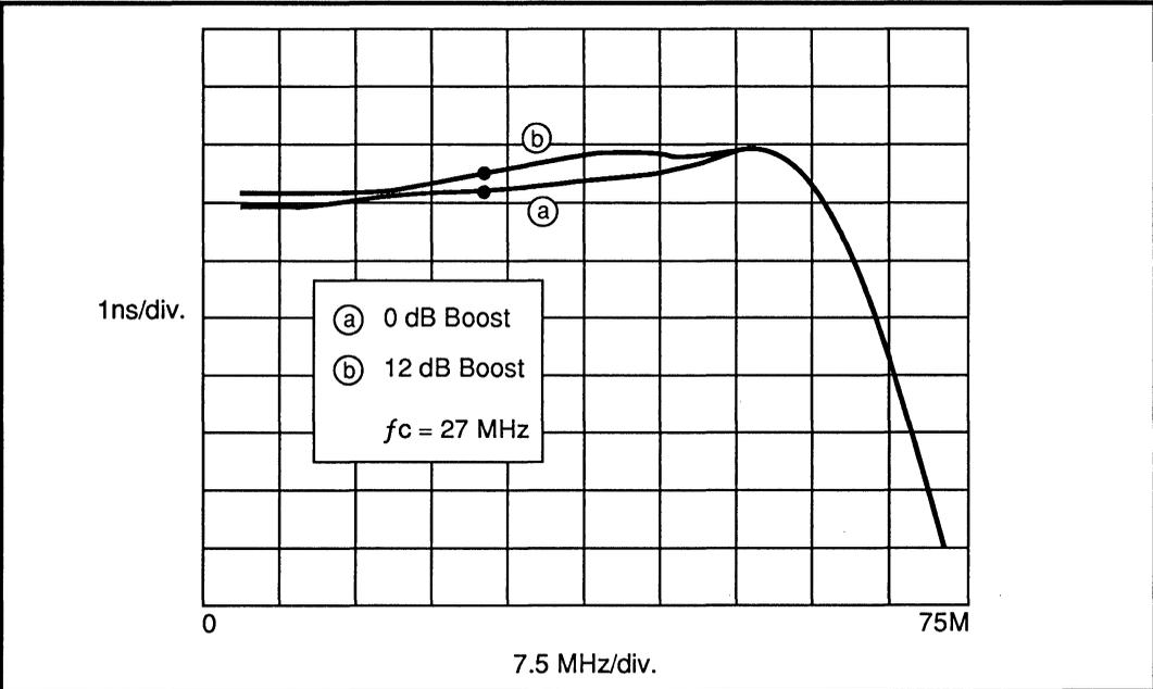
**FIGURE 3: 32F8000 Group Delay Response with  $f_c = 27 \text{ MHz}$**
