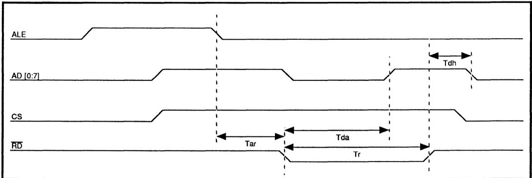
FIGURE 4: Register Read Timing
