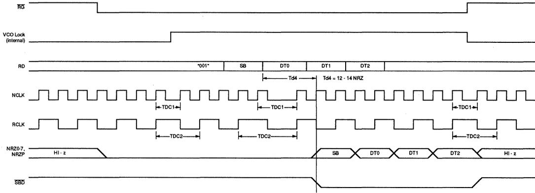
**FIGURE 10: Read Mode NRZ Data Timing**
