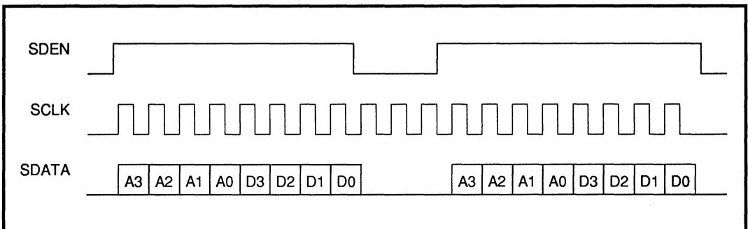
**FIGURE 3: Serial Port Timing, Multiple Transfers**
