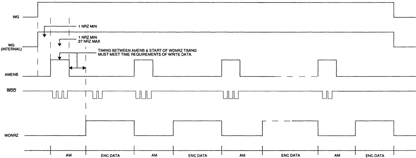
FIGURE 14: Multiple Address Mark Write
