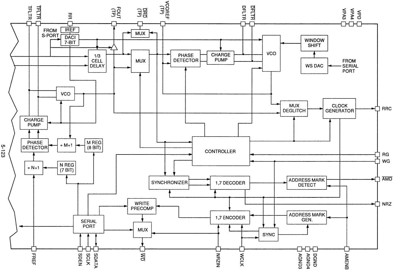
FIGURE 1(B): SSI 32P4730 Combo Device Part 2
