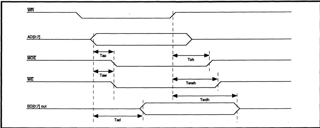
FIGURE 11: Register 70H Write Timing
