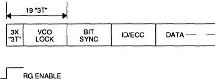
$\overline{AMD}$  remains inactive. A hard sector read operation does not require an address mark search but starts with a preamble search as with soft sector and sequences identically. In all respects, with the exception of the address mark search sequence, hard sector read operation is the same as soft sector read.
