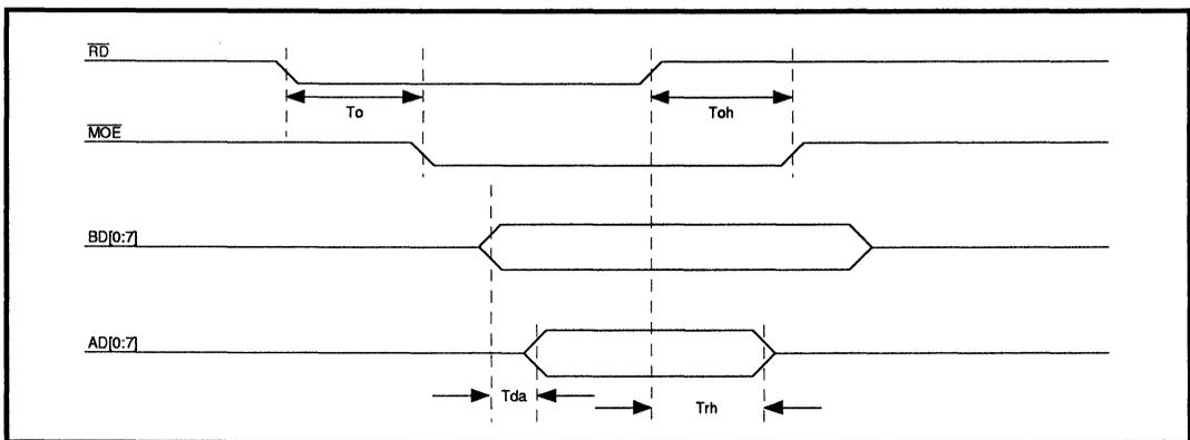
FIGURE 8: Register 70H Read Timing
