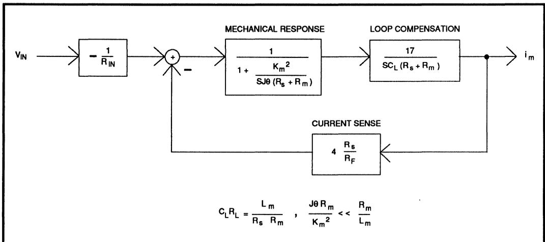
FIGURE 4(B): Simplified Transfer Function Of
