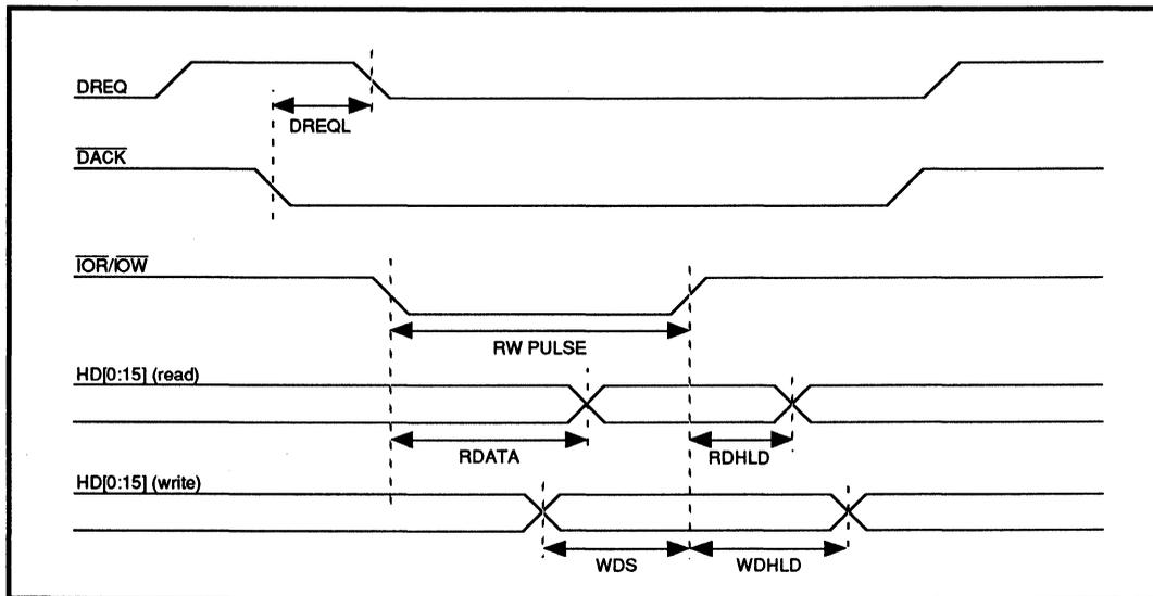
FIGURE 1: Host DMA 8/16-Bit Interface Timing
