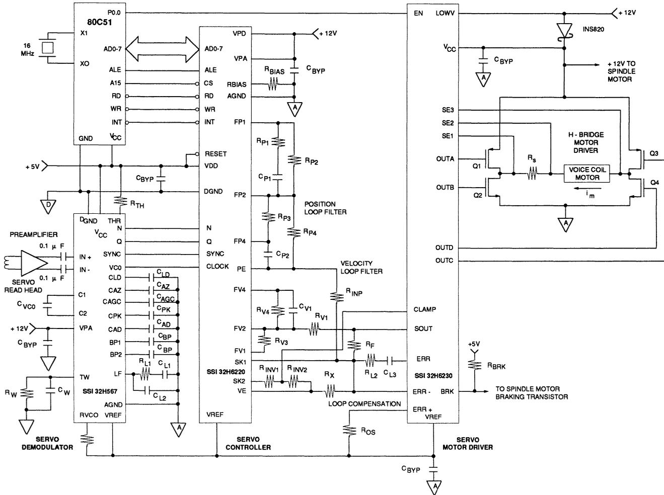
FIGURE 7: Complete Example of Servo Path Electronics Using SSI 32H567/6220/6230 Chip Set
