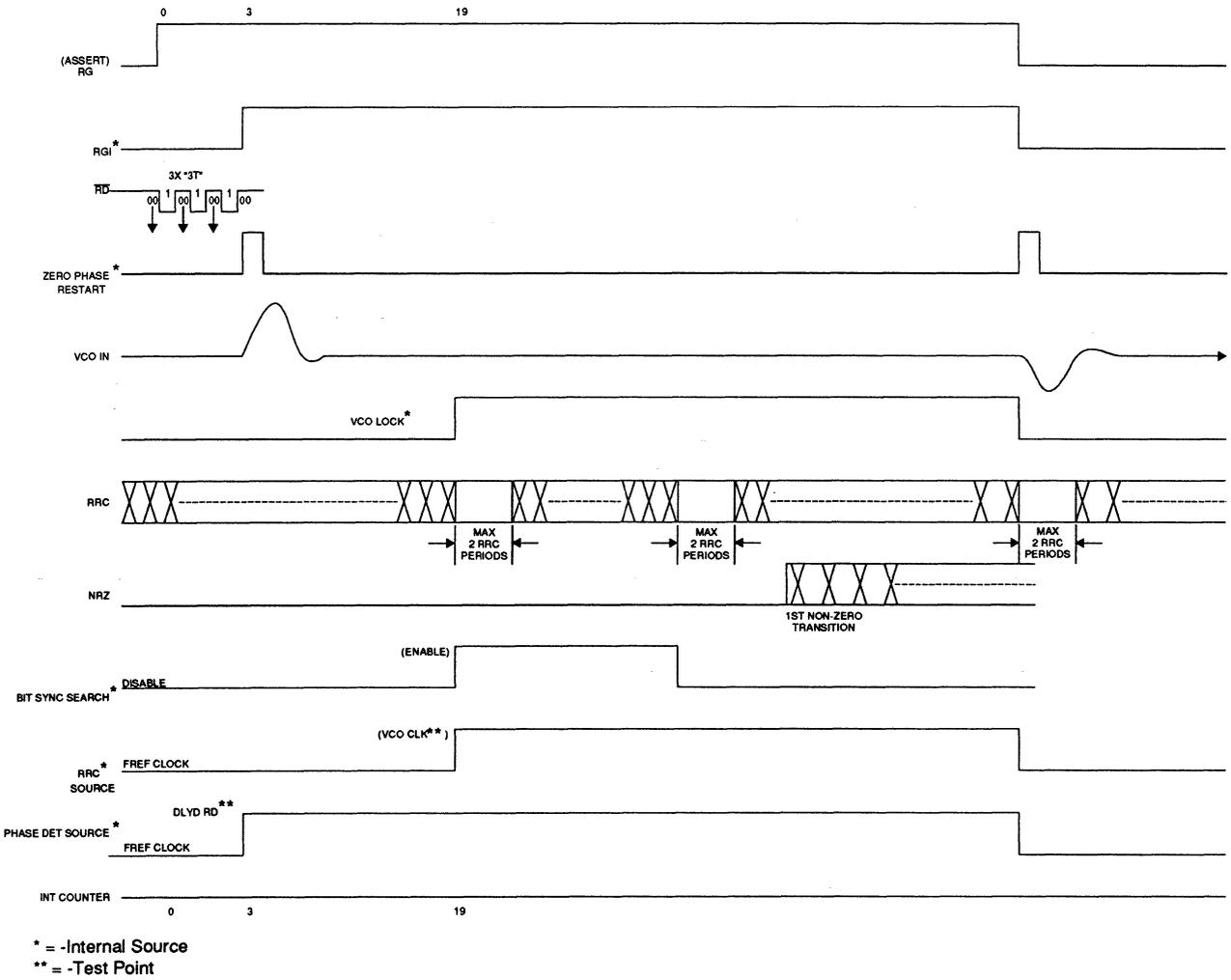
FIGURE 9: Read Mode Locking Sequence (Soft and Hard Sector)
