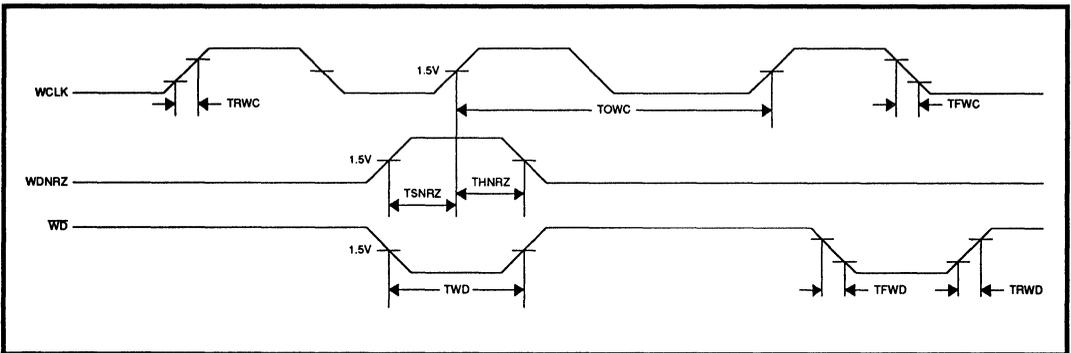
**FIGURE 5: Write Timing**
