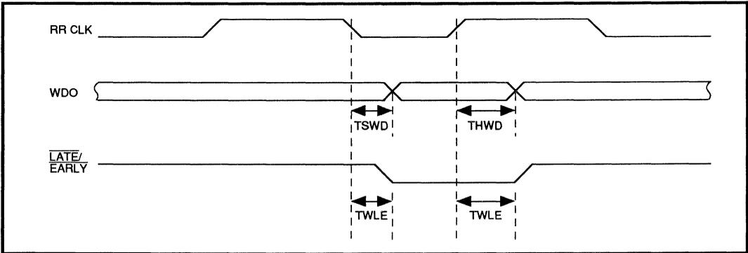
**FIGURE 11 : Write Data Timing - RLL ENDEC Mode**
