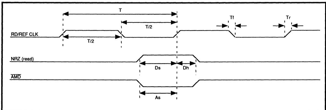
**FIGURE 5: Disk Read Timing**
