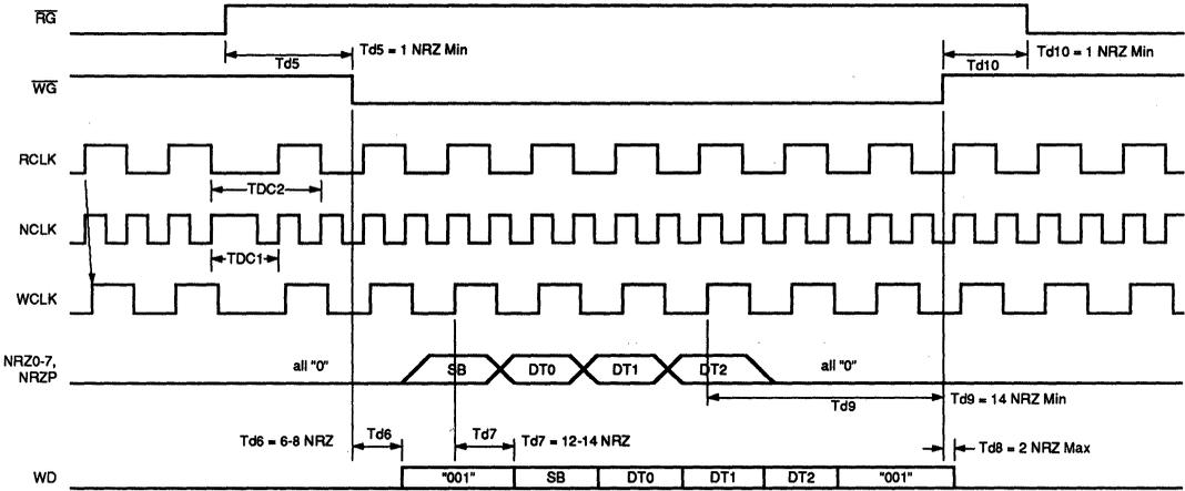
**FIGURE 13: Write Mode NRZ Timing**
