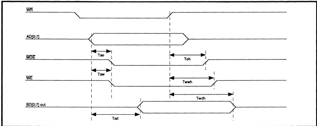
**FIGURE 9: Register 70H Write Timing**
