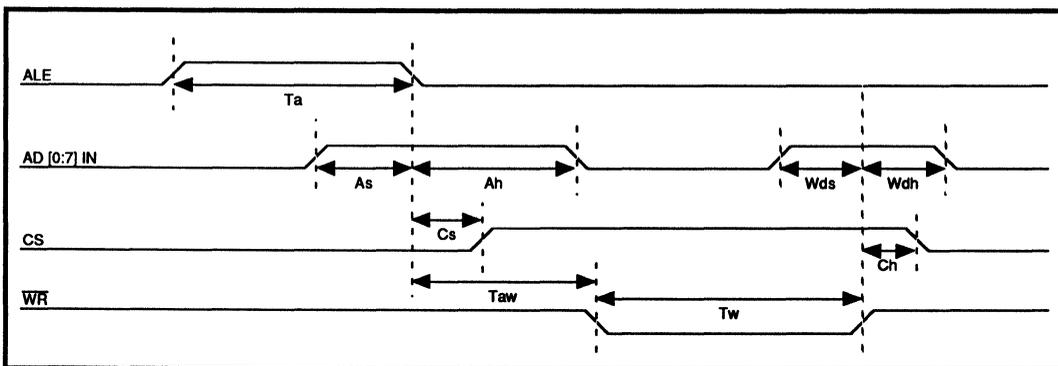
FIGURE 5: Register Write Timing
