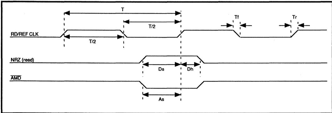
FIGURE 8: Disk Read Timing
