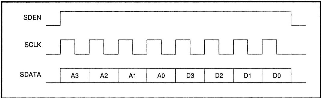
FIGURE 2: Serial Port Timing
