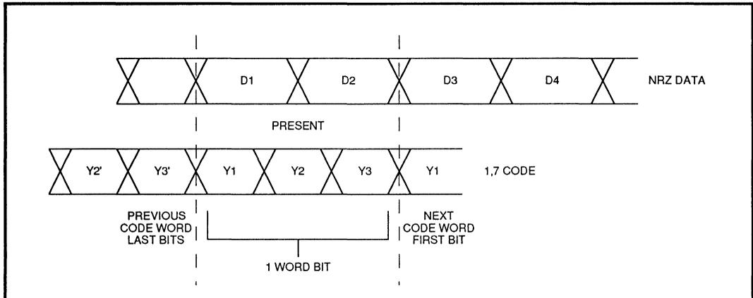
FIGURE 4: NRZ Data Word Comparison to 1, 7 Code Word Bit (See Table 1, for Decode Scheme)
