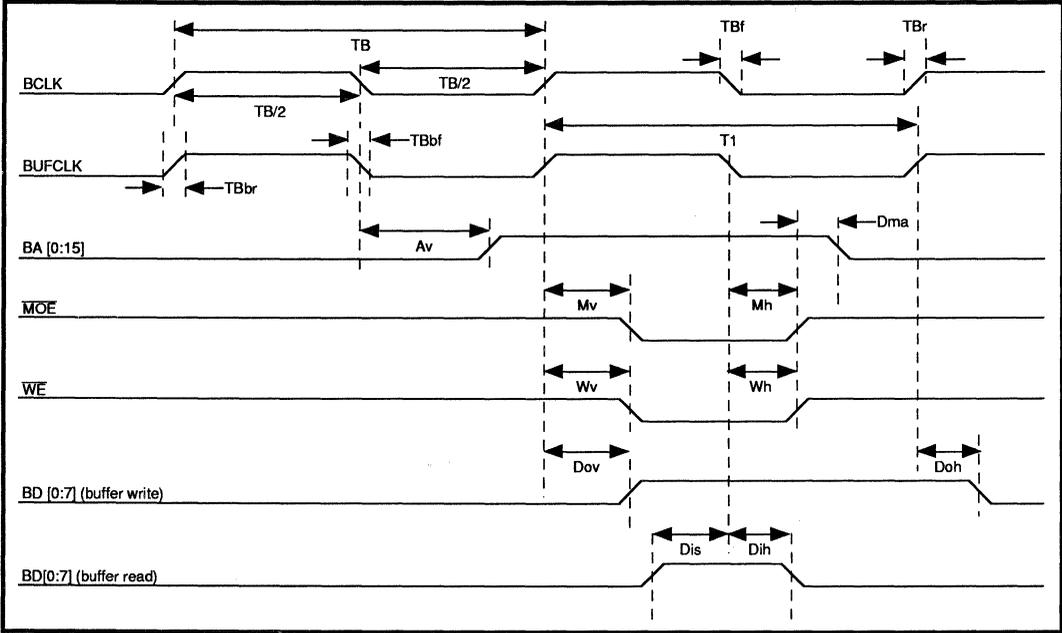
**FIGURE 9: Buffer Memory Read/Write Timing**
