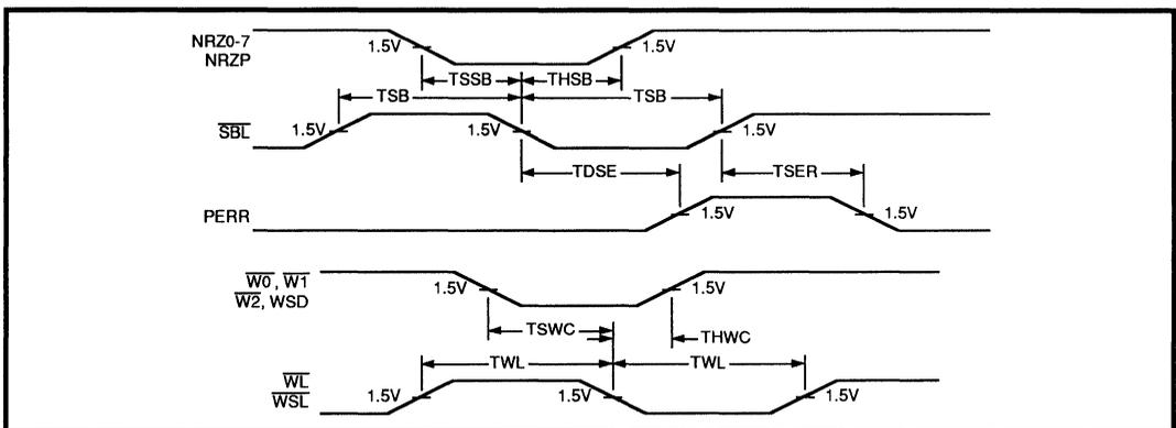
FIGURE 7: Control Timing
