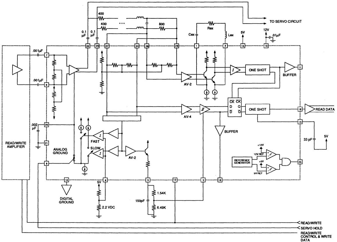
NOTE: Circuit traces for the 12V bypass capacitor and the AGC Hold Capacitor should be as short as possible with both capacitors returned to the Analog Ground Pin.
