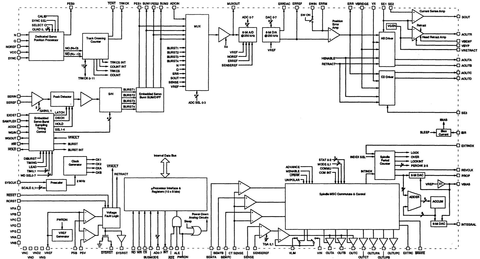
FIGURE 1: SSI 32H4631 Block Diagram
