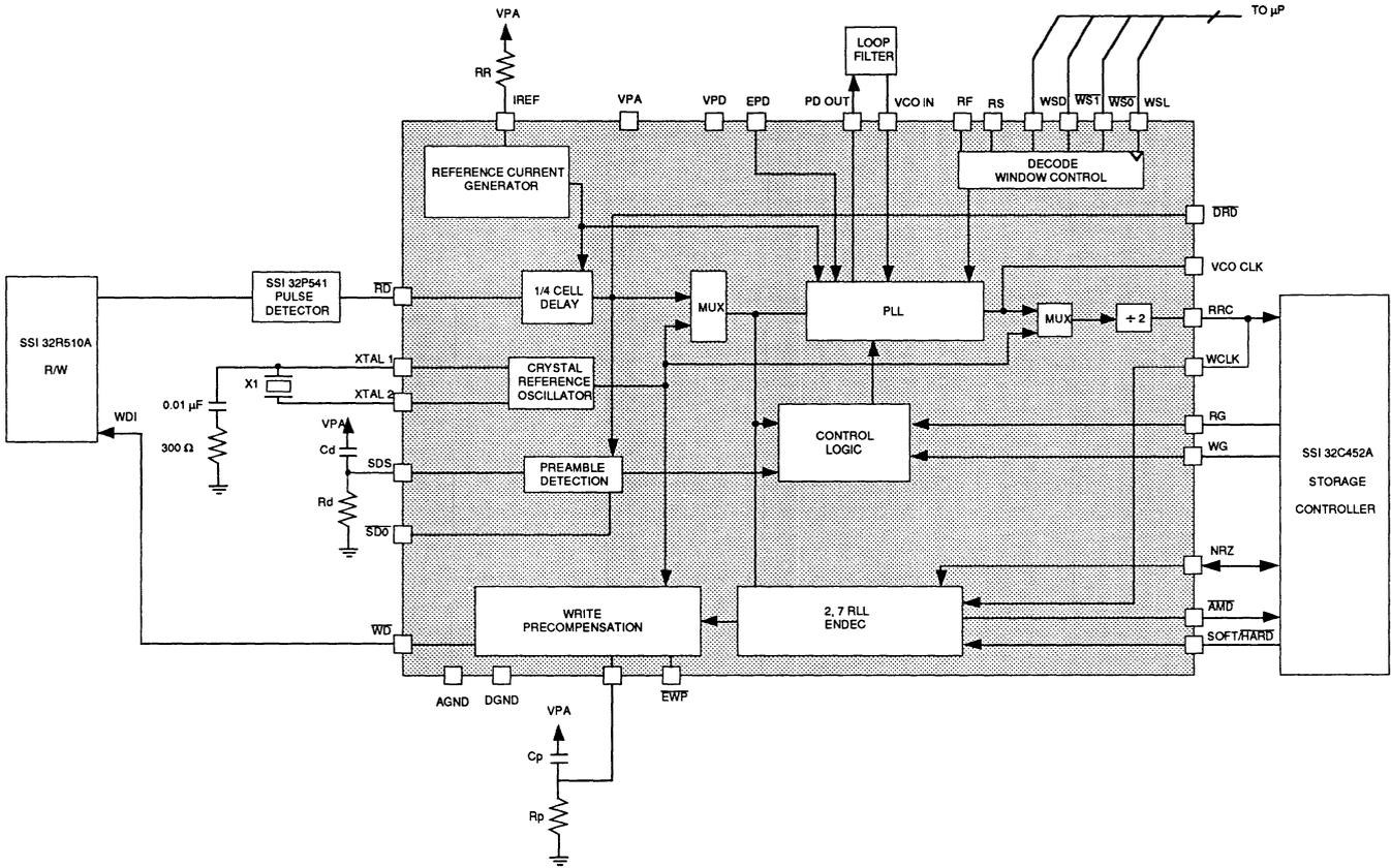
FIGURE 13: Typical SSI 32D5351A Application
