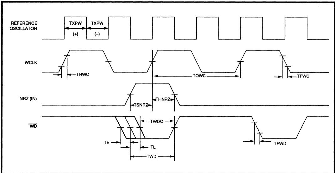
**FIGURE 10: Write Timing**
