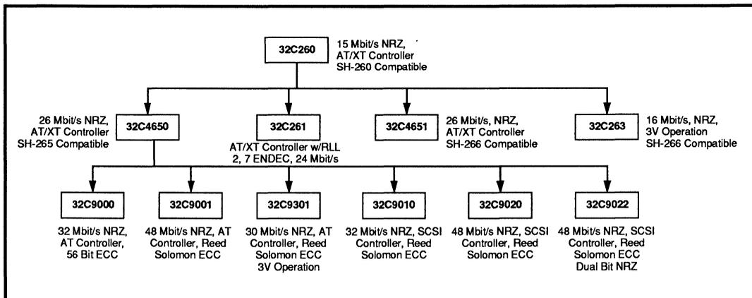
FIGURE 1: Silicon Systems' Disk Controller Chip Hierarchy
