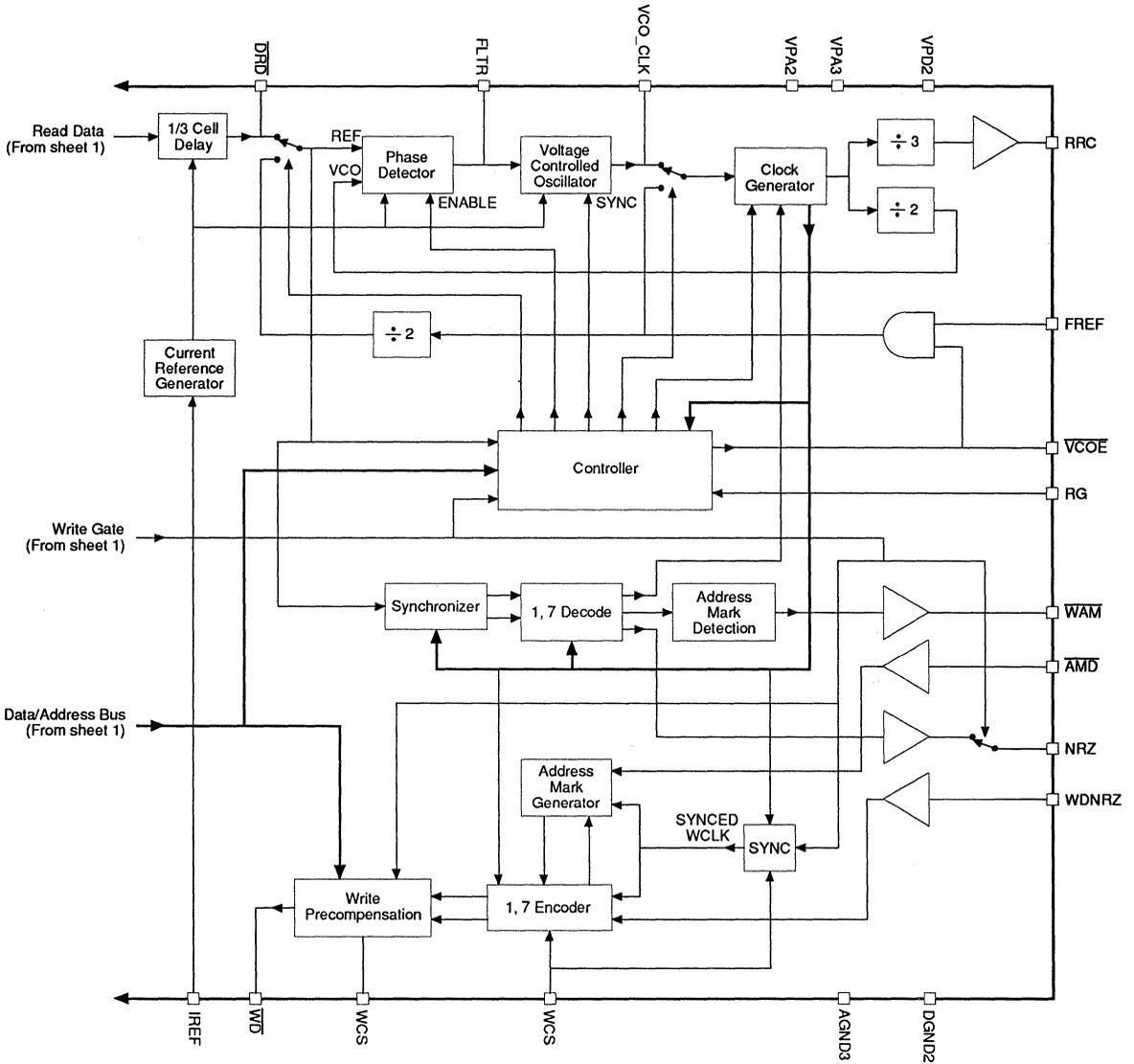
FIGURE 5b: SSI 32P4622 Circuit Block Diagram (Sheet 2)
