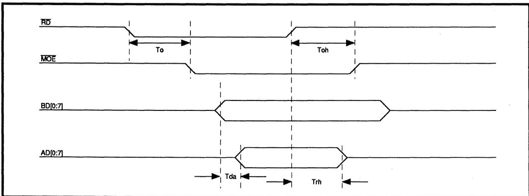
FIGURE 7: Register 70H Read Timing
