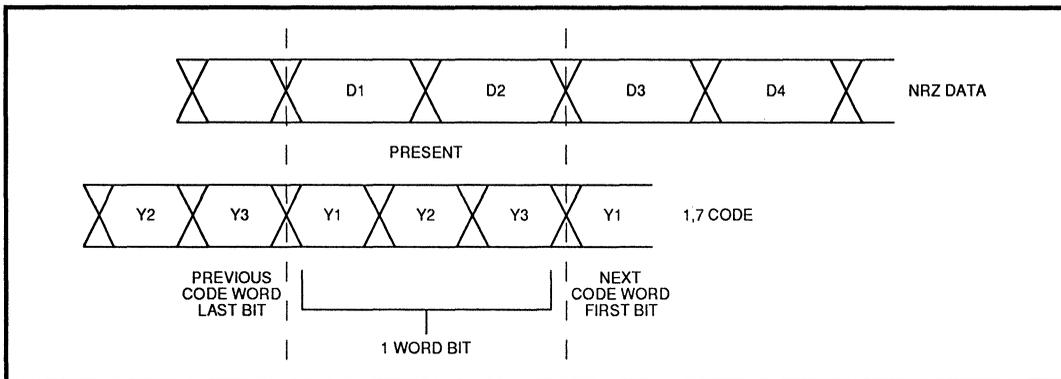
FIGURE 9: NRZ Data Word Comparison to 1, 7 Code Word Bit
