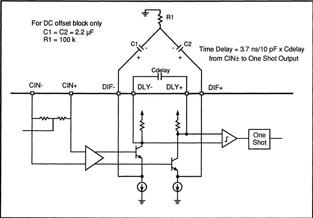
FIGURE 4: SSI 32P5411B Clock Delay Application Diagram
