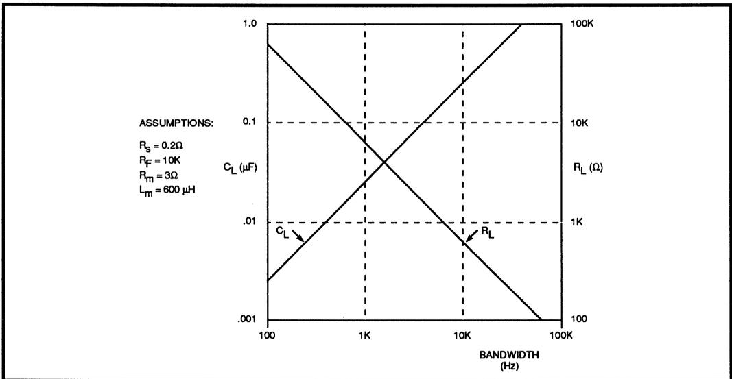
**FIGURE 6: Typical Motor Driver Compensation**
