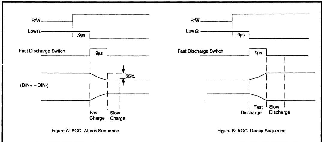
**FIGURE 6: AGC Timing Diagram**
