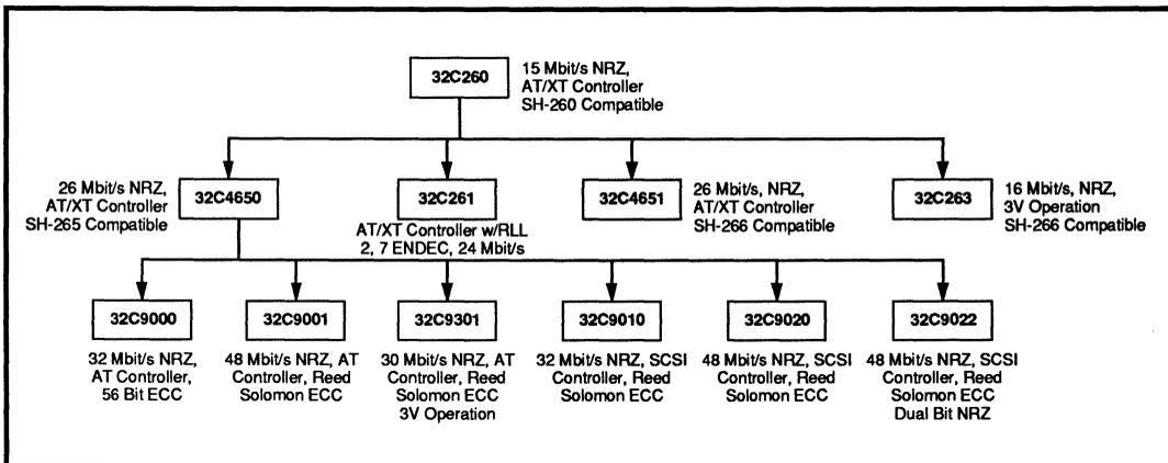
FIGURE 1: Silicon Systems' Disk Controller Chip Hierarchy
