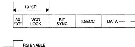
In hard sector operation a low AMENB disables the SSI 32D537X's Address Mark Detection circuitry and  $\overline{AMD}$  remains inactive. A hard sector read operation does not require an address mark search but starts with a preamble search as with soft sector and sequences identically. In all respects, with the exception of the address mark search sequence, hard sector read operation is the same as soft sector read.
