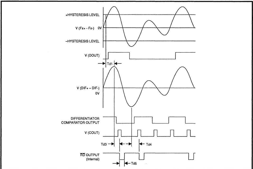
FIGURE 7: Read Mode Digital Section Timing Diagram
