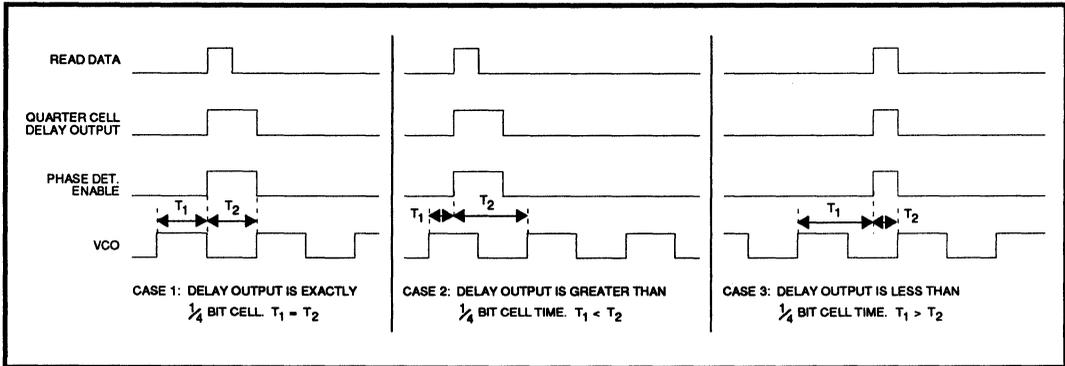
**FIGURE 15B: Timing of Phase Detector Enable Logic.** The read data input pulse can shift to the left by  $T_1$  and to the right by  $T_2$  before an error occurs in the phase detector output polarity, If the quarter cell delay output is not exactly 1/4 bit cell wide, then  $T_1 \neq T_2$ , as shown in cases 2 and 3.
