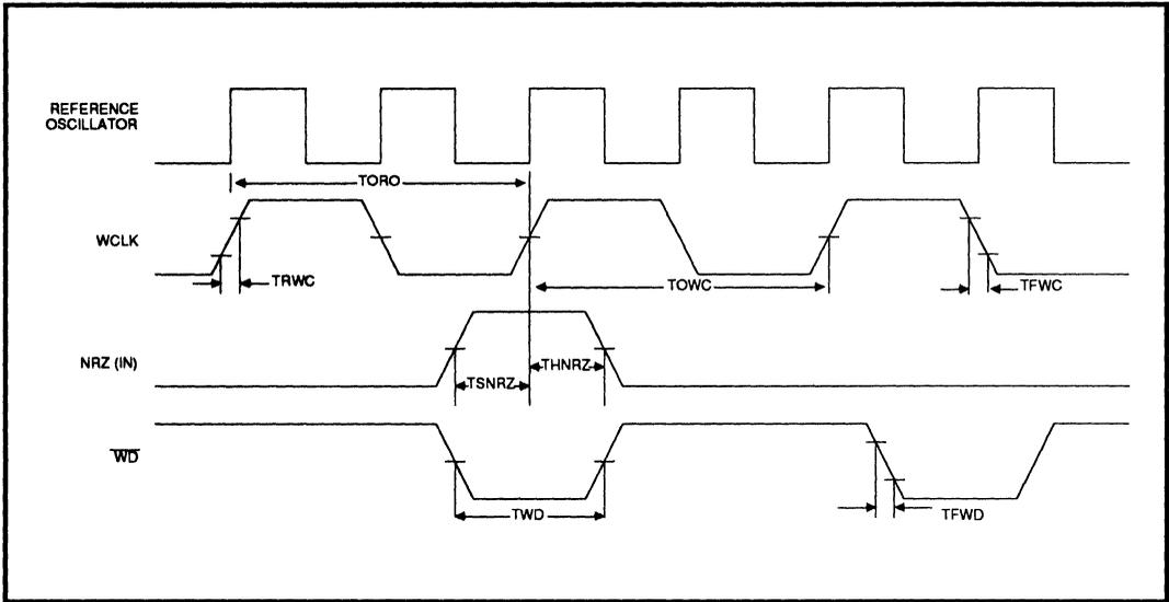
FIGURE 10: Write Timing
