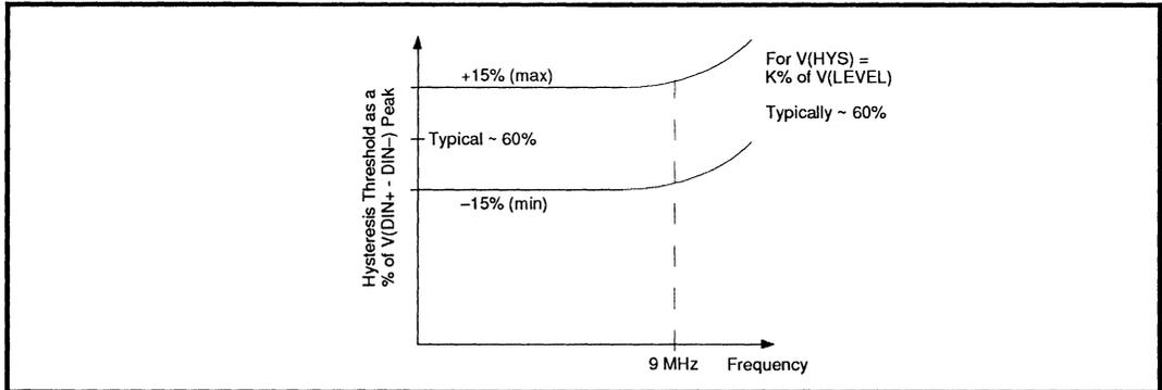
FIGURE 18: Percentage Threshold vs. Frequency
