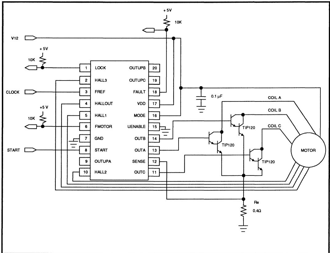
**FIGURE 5: Typical Three-Phase, 8-Pole, Unipolar,
