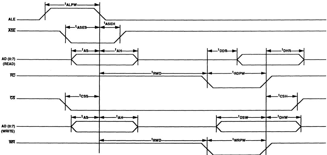
FIGURE 5: Intel Microprocessor Bus Interface Timing Diagram
