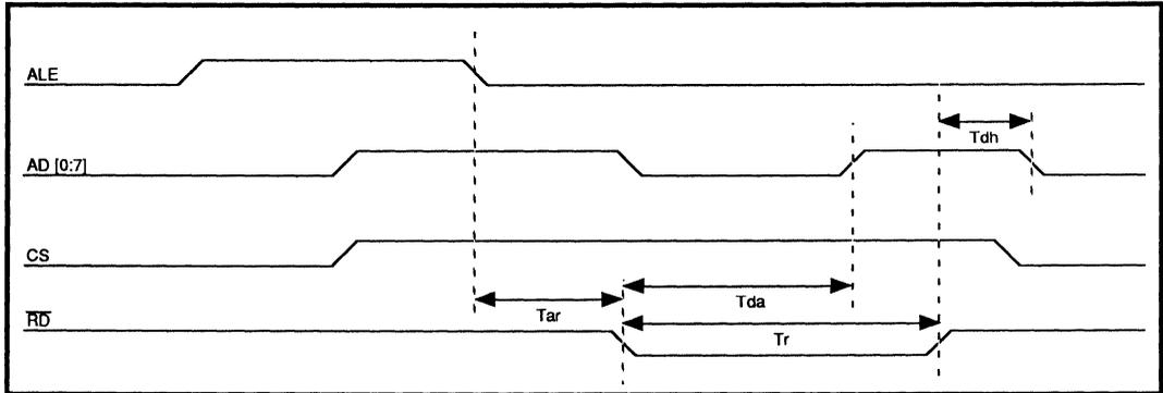
**FIGURE 4: Register Read Timing**
