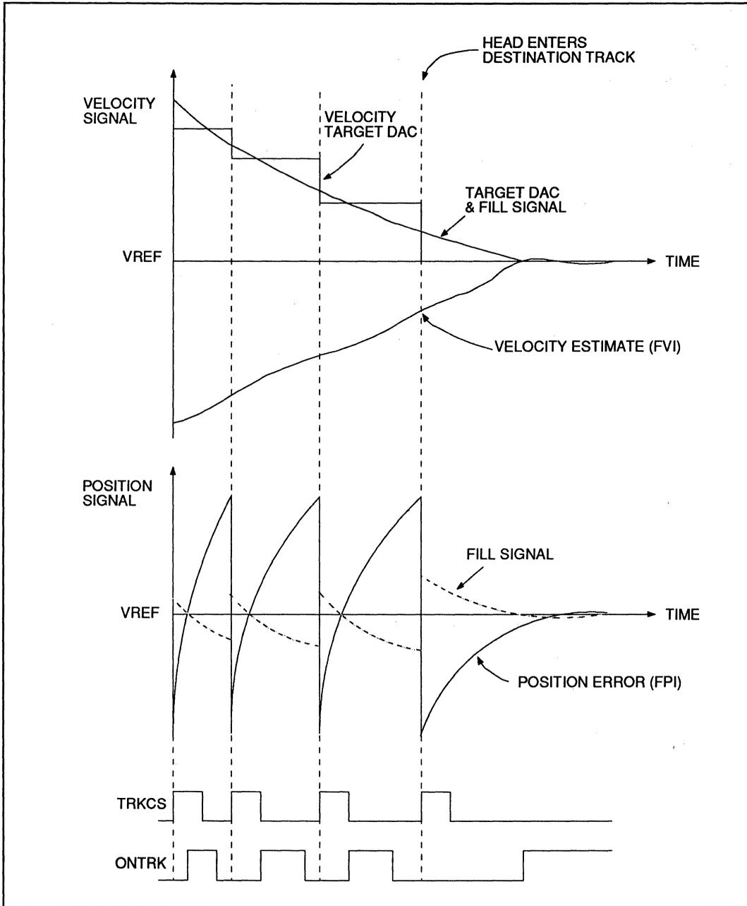
FIGURE 9: Typical Waveforms During Final Deceleration Mode
