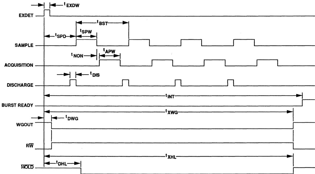
FIGURE 3: Embedded Servo Timing Diagram with Internal Timing Source
