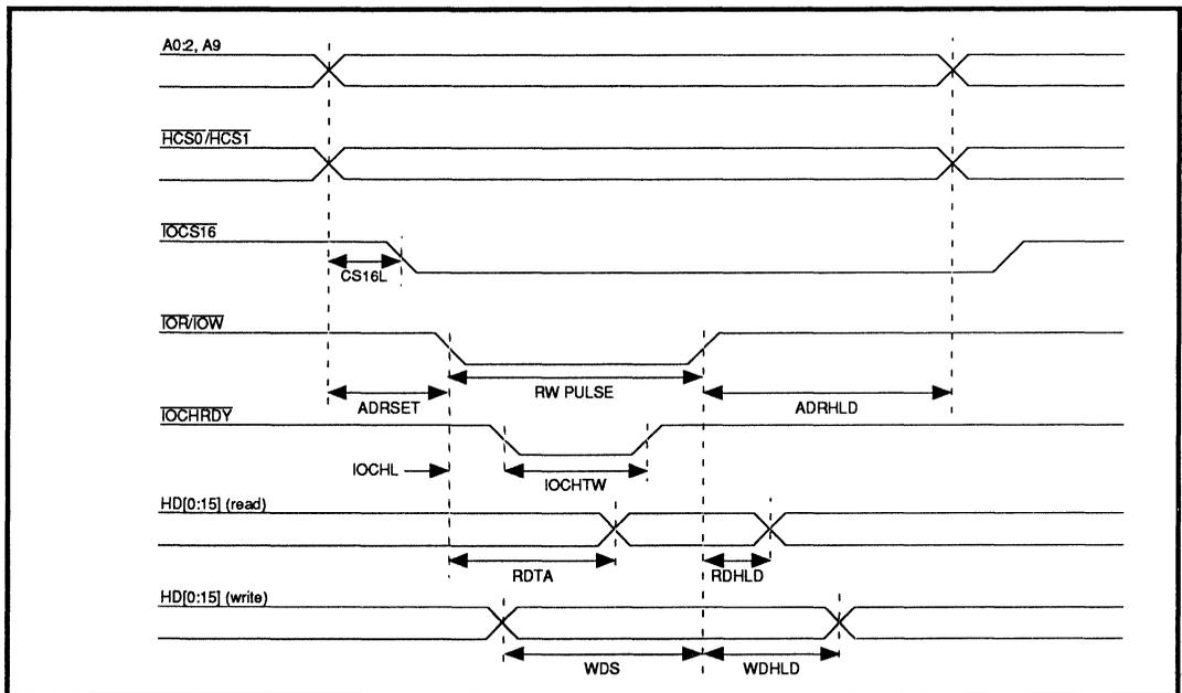
**FIGURE 2: Host Programmed 8/16-Bit Timing**
