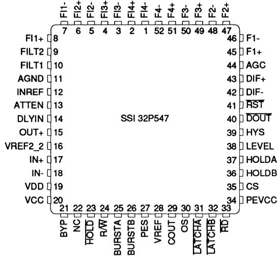
52-Pin Ledged Chip Carrier
