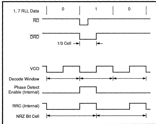
**FIGURE 3: Data Synchronization Waveforms**
