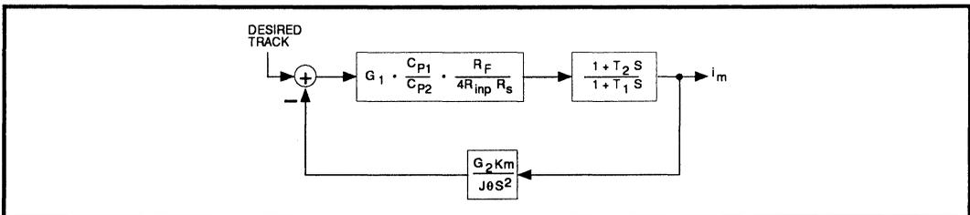
FIGURE 8(b): Simplified Track Mode Transfer Function
