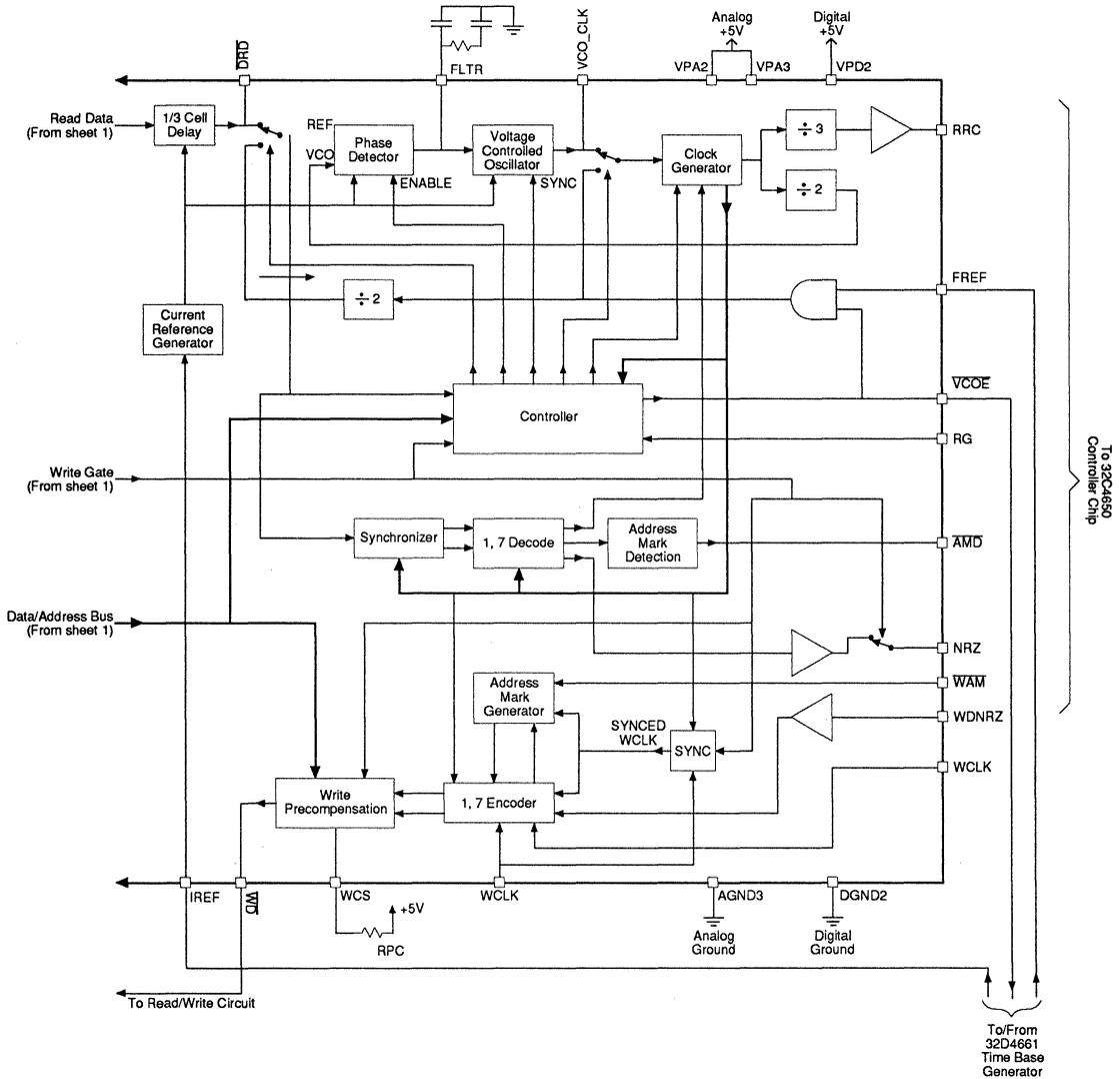
FIGURE 17b: SSI 32P4622 System Configuration (Sheet 2)
