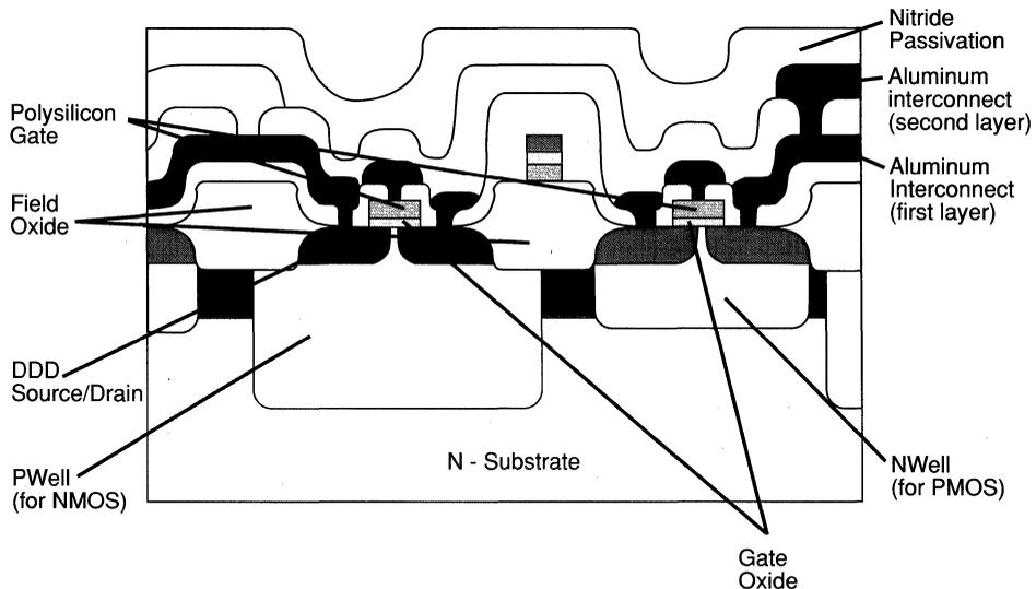
FIGURE 1: CG CMOS Process Transistor
