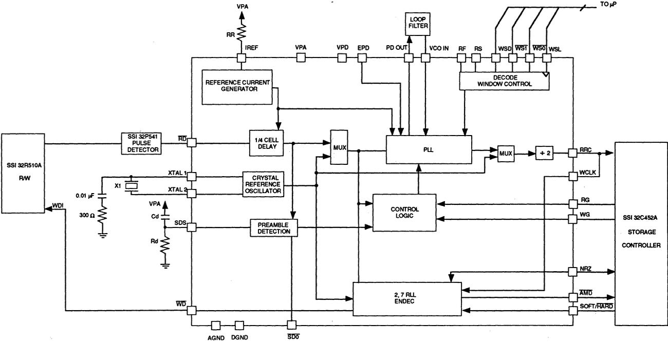
**FIGURE 12: SSI 32D5322 Typical Application**
