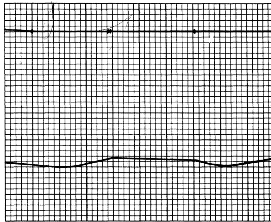
Fig. 203 - DC output-voltage waveform ( t=5 \mu\text{s}/\text{div.} ).
