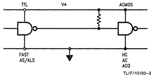
FIGURE 3-2.  $V_{IH}$  Pull-Up on TTL Outputs
