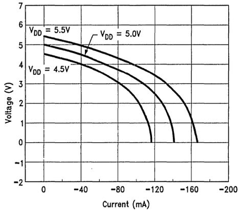
FIGURE 1-4b. Output Characteristics
