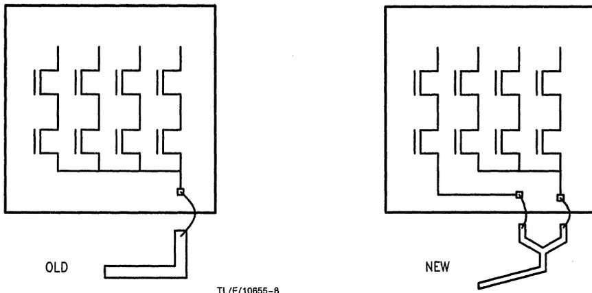
FIGURE 8. Split Ground Bus Structure
