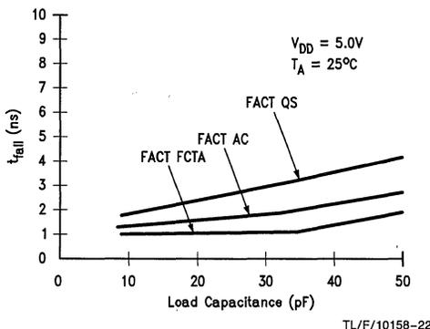
FIGURE 1-15.  $t_{fall}$  vs Capacitance
