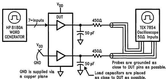
FIGURE 13. Simultaneous Switching Test Circuit
