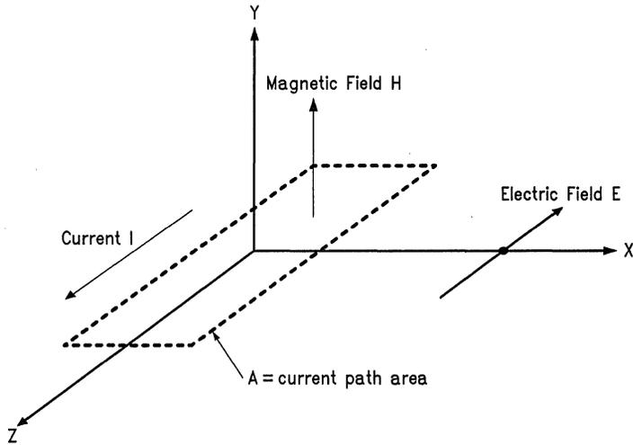
**FIGURE 3-16. EMI is Generated by a Current Flowing along Some Path (Loop)**
