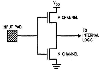
FIGURE 3-19. CMOS Input Structure
