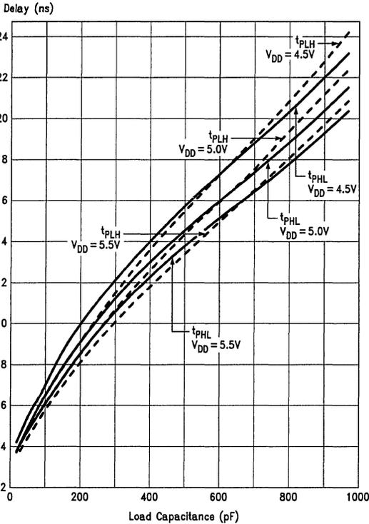
**FIGURE 1-13b. Propagation Delay vs  $C_L$  ('ACTQ244)**
