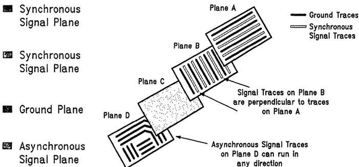
FIGURE 3-11a. Recommended Crosstalk—Avoidance Structure
