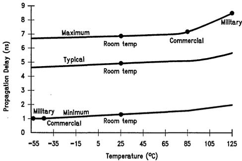
FIGURE 1-11g.  $t_{pHL}$ , 'AC244, with Voltage and Process Variation TL/F/10158-18
