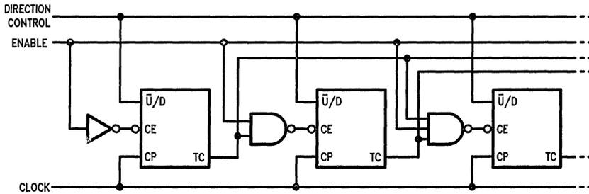
**FIGURE C. Synchronous N-Stage Counter with Parallel Gated Carry/Borrow**
