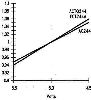
FIGURE 1-11e. Voltage Effects on Delay Times TL/F/10158-16
