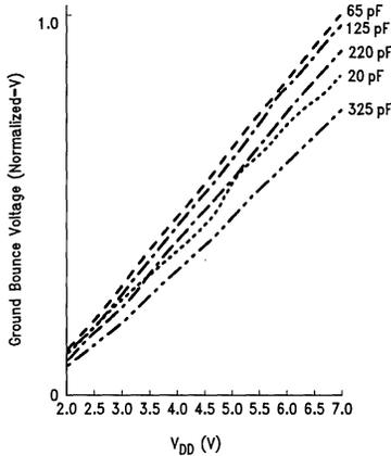
FIGURE 20. Quiet Output Noise vs Power Supply
