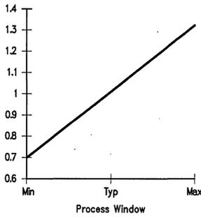
FIGURE 1-11f. FACT Process Effects on Delay Times TL/F/10158-17
