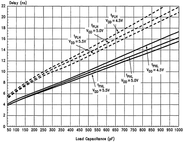
**FIGURE 1-13a. Propagation Delay vs  $C_L$  ('AC00)**
