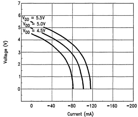
FIGURE 1-4c. Output Characteristics
