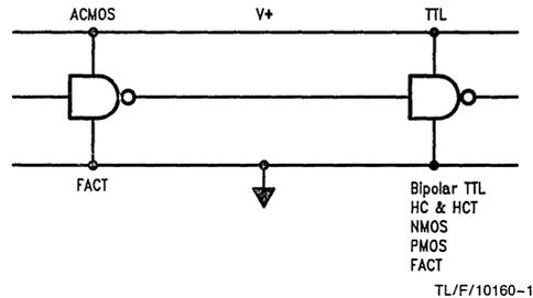
FIGURE 3-1. Interfacing FACT to NMOS, CMOS, and TTL
