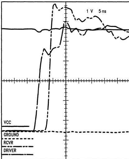
**FIGURE 3. Effects of Input Clamp Diodes
