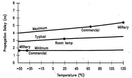
FIGURE 1-11i.  $t_{pHL}$ , 'FCT244A, with Voltage and Process Variation TL/F/10158-34
