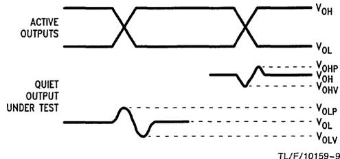
FIGURE 12. Quiet Output Noise Voltage Waveforms
