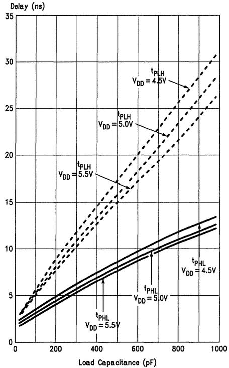
**FIGURE 1-13c. Propagation Delay vs  $C_L$  ('FCT244A)**
