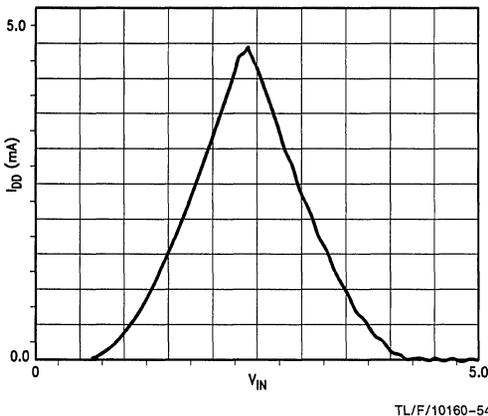
**FIGURE 3-21.  $I_{DD}$  versus  $I_{IN}$  for 'AC Devices**
