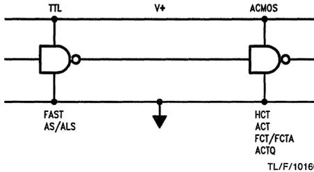
**FIGURE 3-3. TTL Interfacing to 'ACT'**
