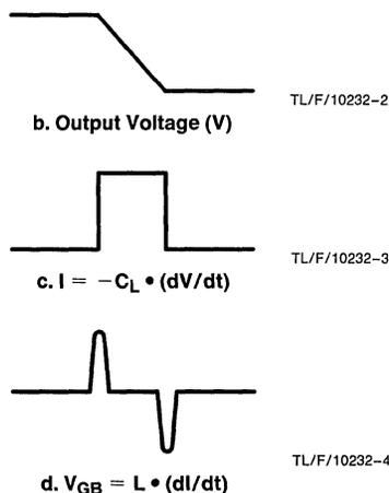
FIGURE 1. Ground Bounce Circuit Model
