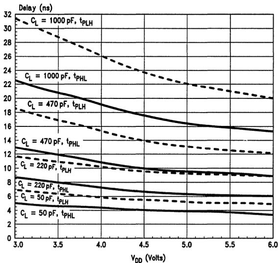
**FIGURE 1-12a. Propagation Delay vs  $V_{DD}$  ('AC00)**
