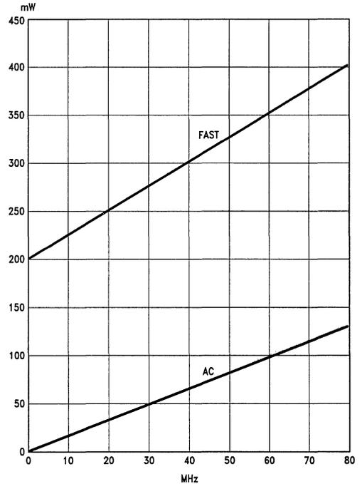
FIGURE 1-10. FACT vs FAST Circuit Power
