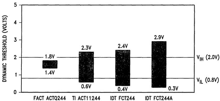
FIGURE 12. AC MOS Dynamic Threshold Comparison
