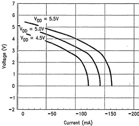
FIGURE 1-4a. Output Characteristics
