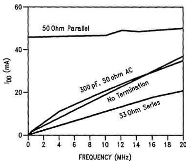
FIGURE 3-6c. FACT  $I_{DD}$  vs Termination
