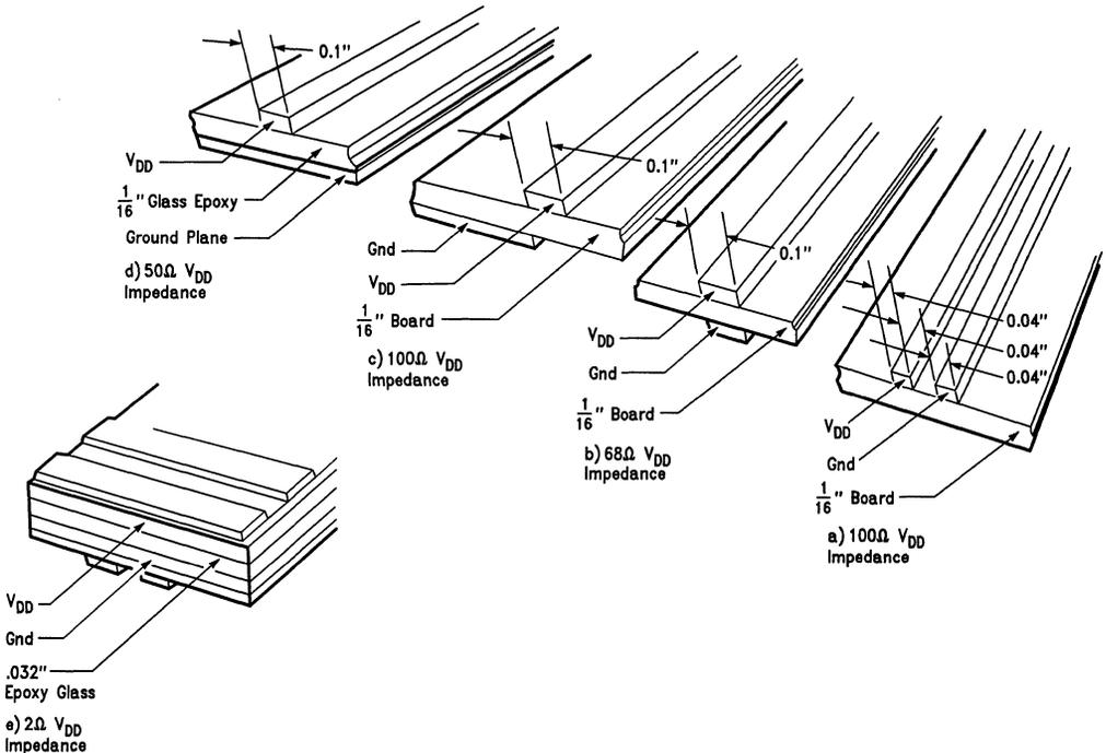
**FIGURE 3-12. Power Distribution Impedances**
