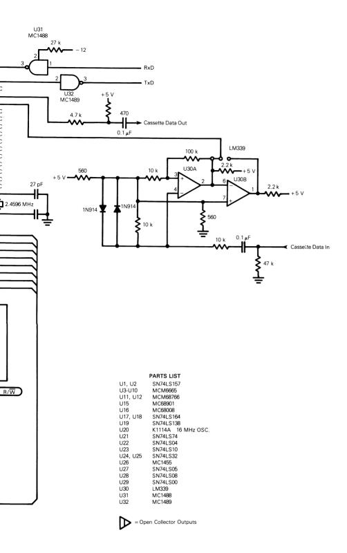
FIGURE 1 — Schematic Diagram of Hardware Used in This Application Note
