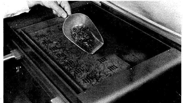
3. Vibrator is turned on and loaded (above) with pins, after a 15 - 30 second cycle 99.9% of the holes have a pin in them (100% fill is common).
