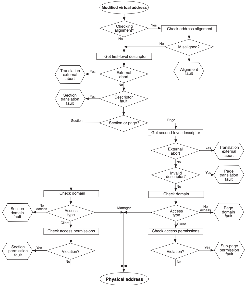
Figure B4-2 Sequence for checking faults
