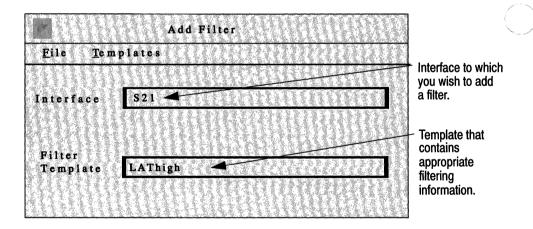
Figure 17-15. Specifying the Appropriate Template and Interface
