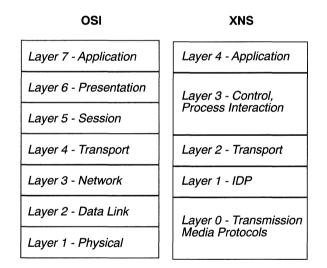
Figure 15-1. Comparison of OSI and XNS Protocol Stacks
