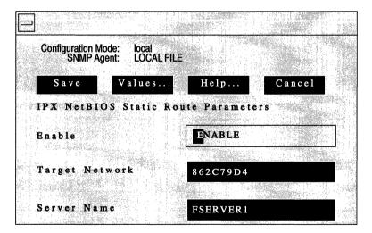
Figure 12-22. IPX NetBIOS Static Route Parameters Window
