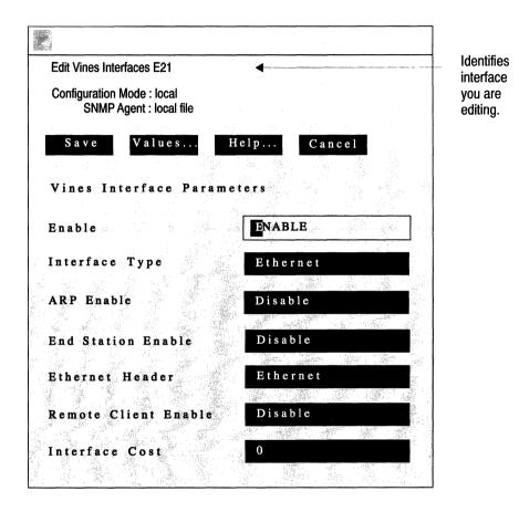
Figure 14-15. VINES Interface Parameters Window
