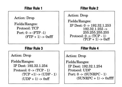
Figure C-4. Example of Version 7 Filters
