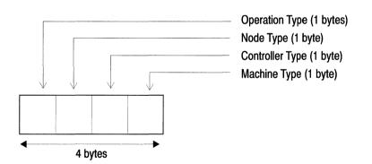
Figure 14-7. VINES Routing Update Protocol Header
