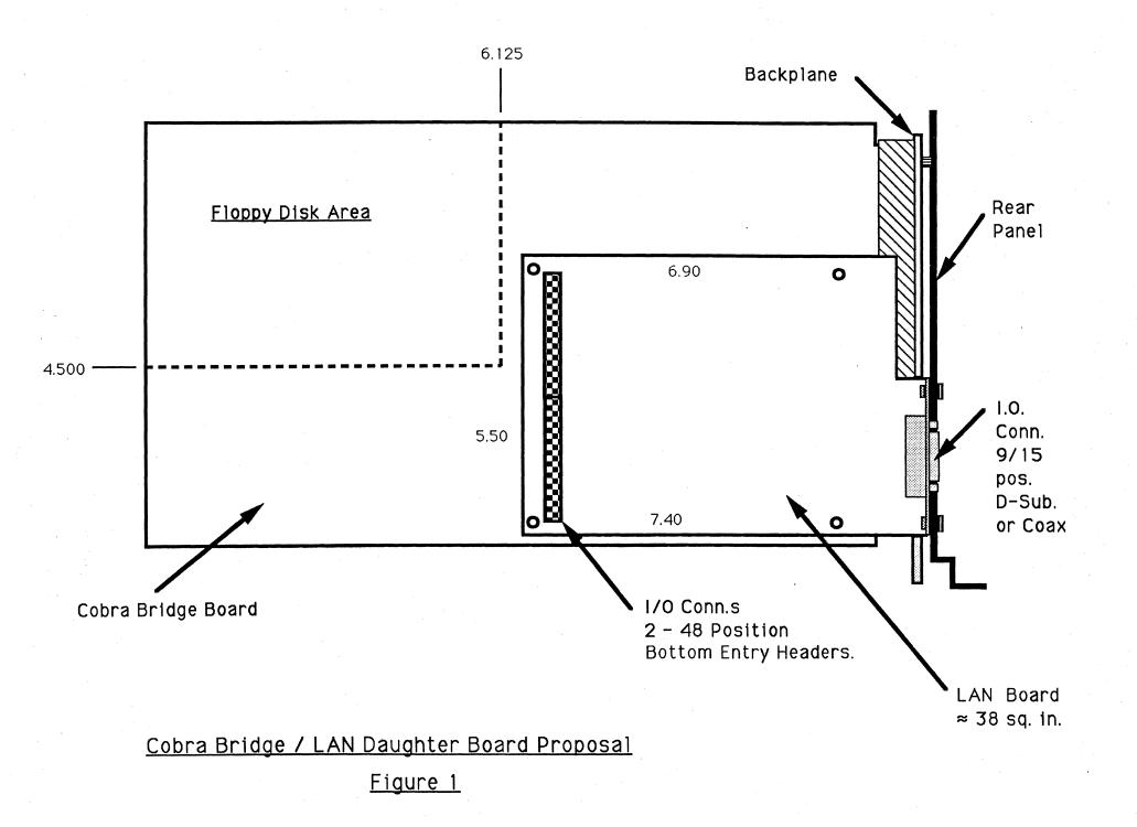
Grounding and mechanical integrity of the Bridge / LAN board are enhanced while stresses imparted to the LAN connector and the daughter board mounting hardware are minimized. Once the LAN connector plate/board is secured to the rear panel with captive hardware the appropriate LAN cable can then be attached. This physical attachment scheme will require that the LAN cable be disconnected from the LAN connector prior to removal of the Main Bridge board/LAN daughter board assembly.
