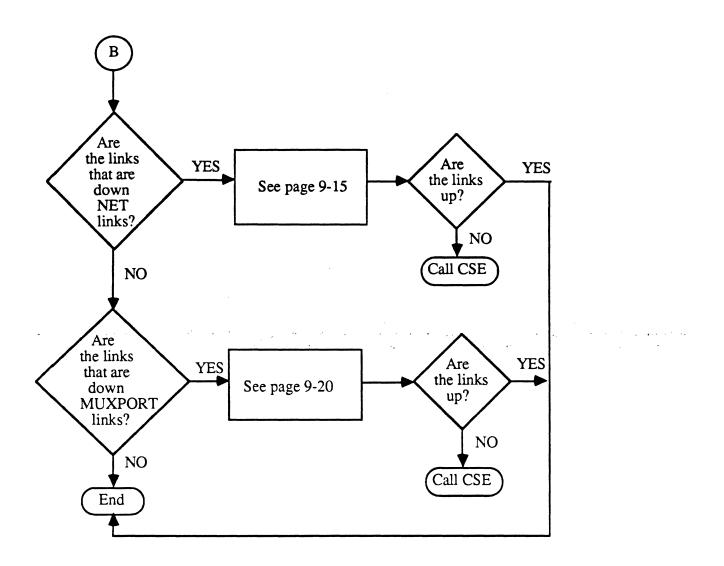
Figure 9-2 (continued). Remote Fault Isolation Flowcharts
