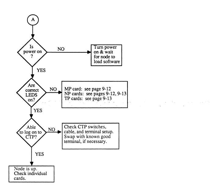
Figure 9-1 (continued). On-Site Fault Isolation Flowcharts
