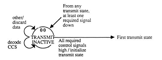
The TRANSMIT INACTIVE state discards all data while one or more of DTR, DSR and DCD are low. The state does process control signal updates and other CCS's coming from the remote end. The control signal handling routines change the transmit state to an active state when all three required signals are up.
