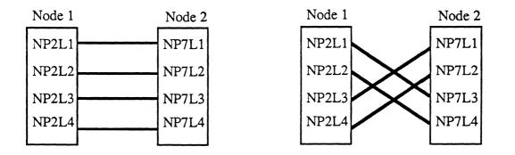
Figure 1-18. Correct Examples of CMMP Group Link Cabling
