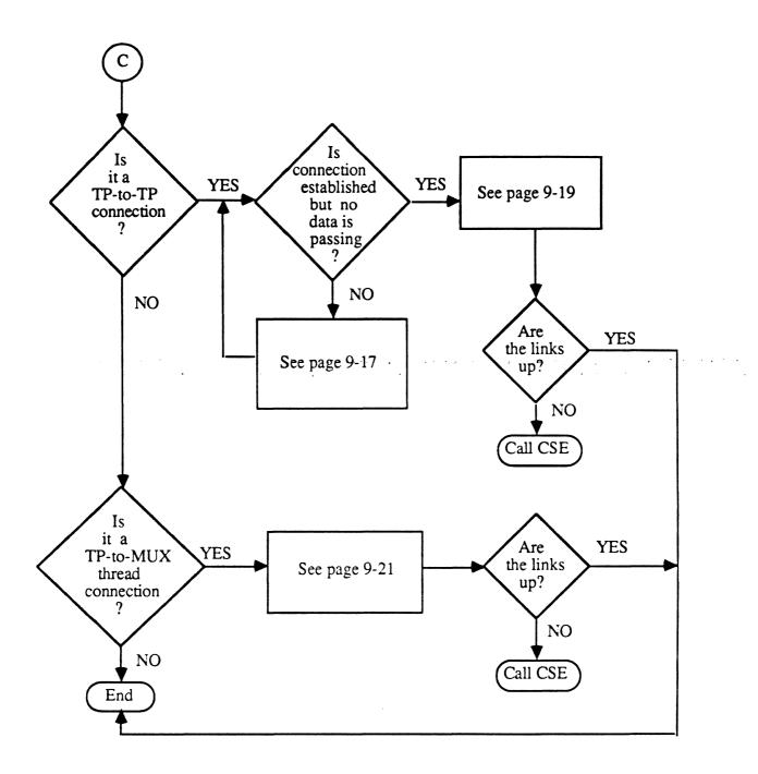
Figure 9-2 (continued). Remote Fault Isolation Flowcharts
