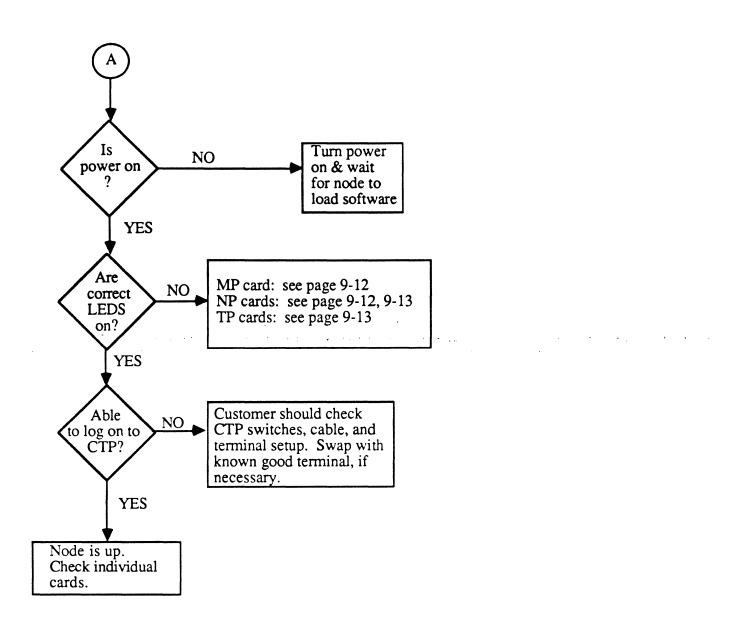
Figure 9-2 (continued). Remote Fault Isolation Flowcharts
