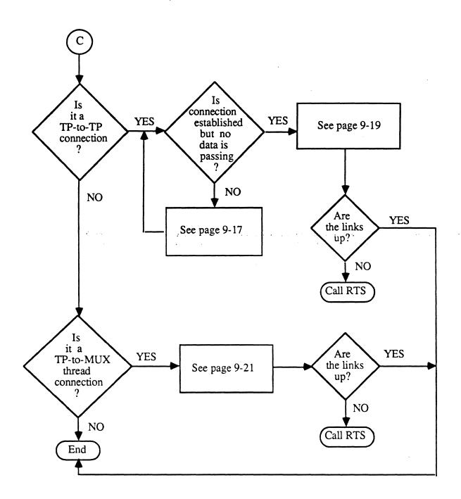
Figure 9-1 (continued). On-Site Fault Isolation Flowcharts
