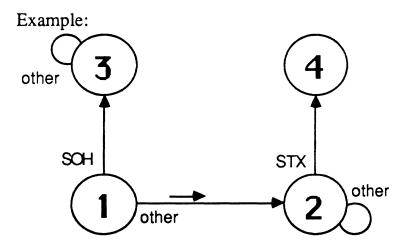
While in state 1, a SOH will be stored in the RXQ (receive side) or sent to the chip (transmit side), and the state will be changed to state 3. With a character other than a SOH we would jump directly from state 1 to state 2, where the character would be stored and the state changed as needed.
