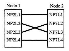
Figure 1-19. Incorrect Example of CMMP Group Link Cabling
