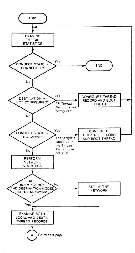
Figure 9-7. TP-to-Muxport Thread Connection - Troubleshooting Flowchart
