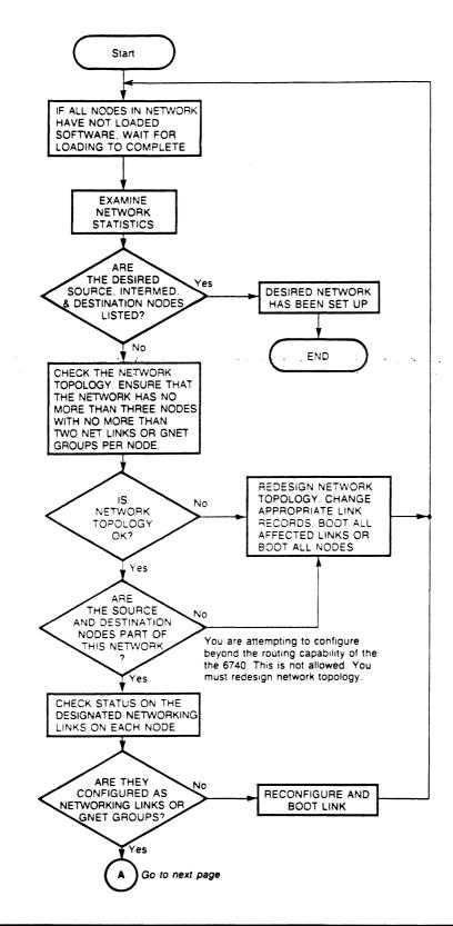
Figure 9-3. Setting Up the 6740 DCP Network - Troubleshooting Flowchart
