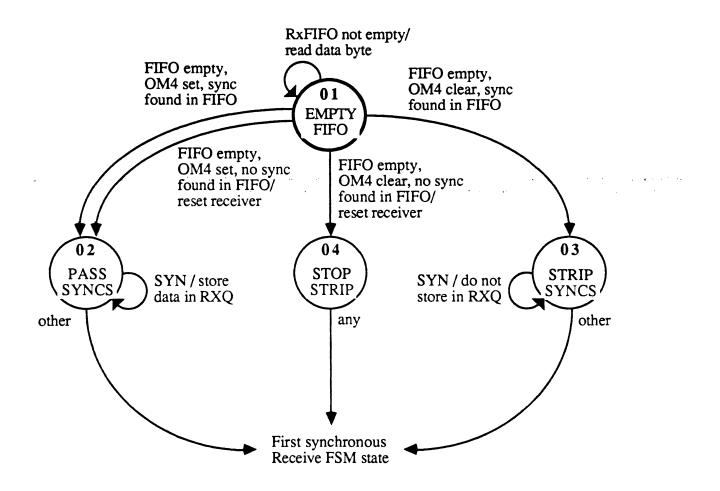
In the EMPTY FIFO state the receive FIFO is emptied, checking for sync characters. If two consecutive syncs are found, or the last character is a sync, then the chip is not reset in case there are no subsequent sync characters for the chip to sync up on. Also, the FSM state is changed to the state which will handle between-message syncs according to the setting of opmode bit 4.
