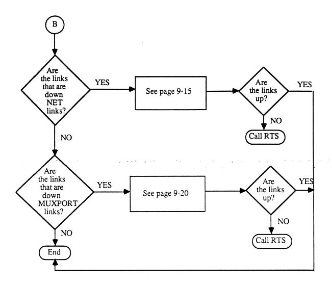
Figure 9-1 (continued). On-Site Fault Isolation Flowcharts
