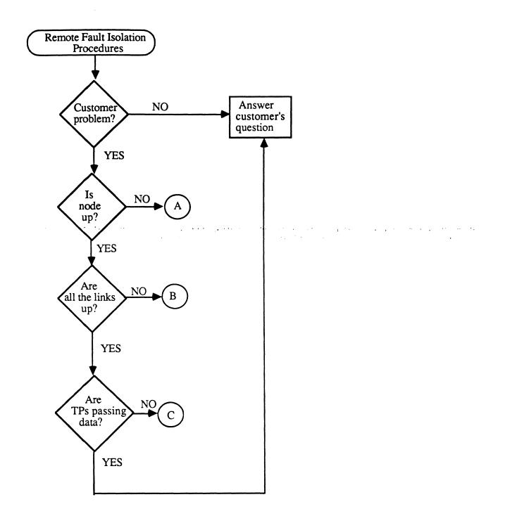
Figure 9-2. Remote Fault Isolation Flowcharts
