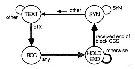
The transition from the last state to the SYN state is caused by the receipt of an end of block CCS. The routine which detects the CCS changes the common state to release the protected characters and perform end of message tasks (e.g. force a pad, drop carrier) and changes the FSM state to SYN.
