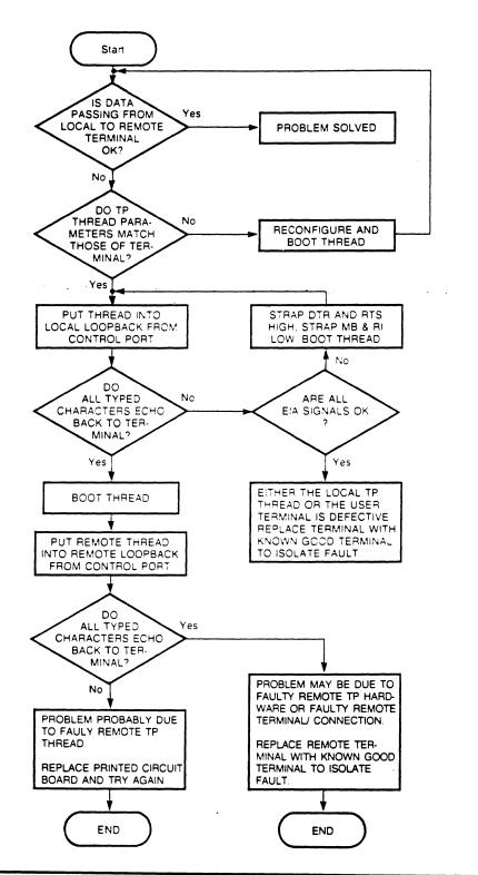
Figure 9-5. TP-to-TP Connection, But No Data Is Passing -Troubleshooting Flowchart
