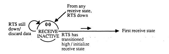
The RECEIVE INACTIVE state handles character interrupts while RTS is low and both DTR and DSR are up. The state checks the current status of RTS upon each interrupt. If the signal is still low, then the data is discarded. If RTS has gone high, then the signal change is acted on, the receive state is changed to an active state and jumped to to process the data byte.
