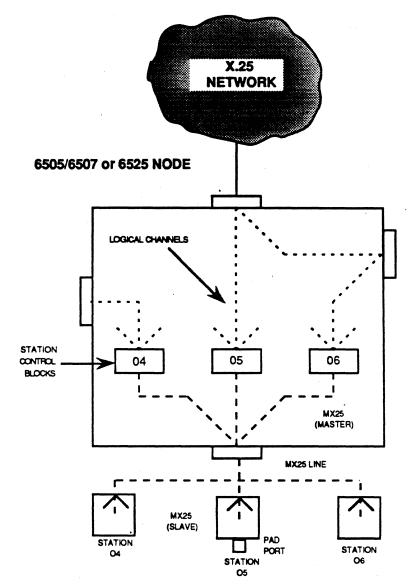
Station xx, where xx is the Station Address on the Multipoint line. Multiple SVCs on an internal Station Contrl Block. SCBs appear as virtual ports with multiple SVCs.
