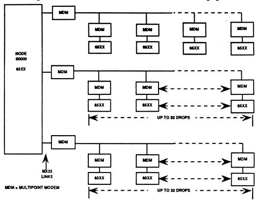
Multipoint X.25 (MX25) is a synchronous, bit-oriented protocol. Up to 256 stations can be defined, with a maximum of 32 stations per MX25 port. All drops on a MX25 port must be full-duplex. Some possible configurations are:
