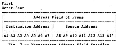
Fig. 2 -- Nonrepeater Address-Field Encoding
