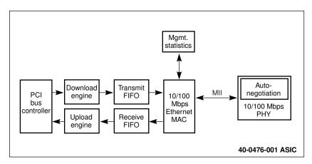
Figure 17 3C905B-TX NIC—40-0483-00x ASIC Block Diagram
