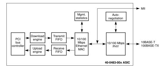
Mgmt. statistics Autonegotiation 10BASE-T/AUI Download Transmit 100 Mbps 10/100 engine FIFO PCI Mbps signaling bus Ethernet controller Upload Receive MAC **FIFO** MII engine control 40-0502-004 ASIC
