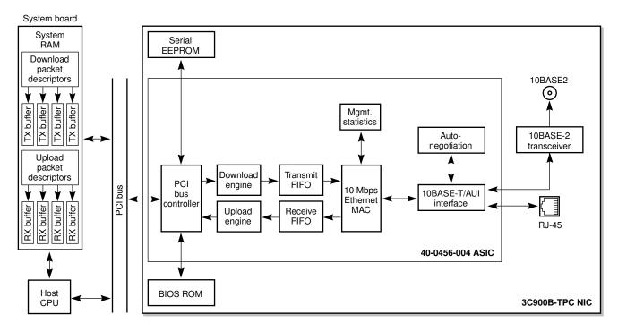
Figure 7 3C900B-COMBO System Architecture
