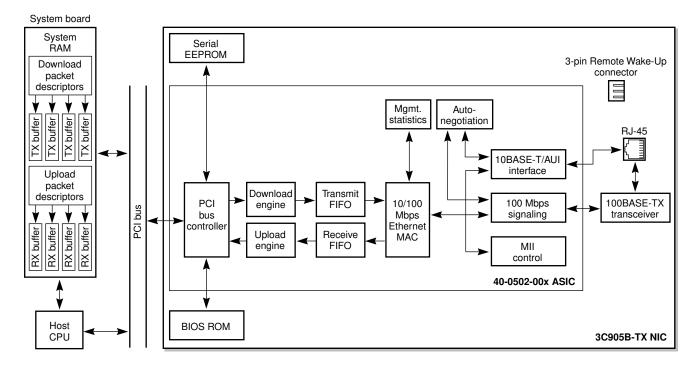
Figure 8 3C905B-TX with 40-0502-00x ASIC System Architecture
