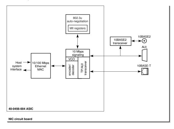
Figure 22 3C900B NICs (40-0456-004 ASIC) Media Port Architecture
