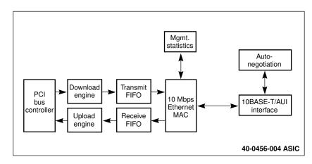
Figure 15 3C905B-TX NIC—40-0502-00x ASIC Block Diagram
