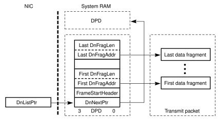
The packet to be transmitted is first placed in data fragments (buffers) in system memory. Next, a list of DPDs (the downlist) that points to the fragments is also created in system memory.
