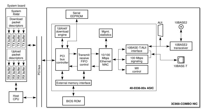
Figure 3 3C905-TX System Architecture
