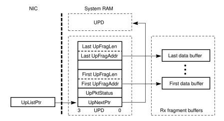
The head of the uplist is the UPD that corresponds to the current upload packet. The Up List Pointer (UpListPtr) register points to this UPD. As the UPD is processed, the fragment address and fragment length values are fetched one by one from the UPD into on-NIC registers, which are used to control the data upload operations.
