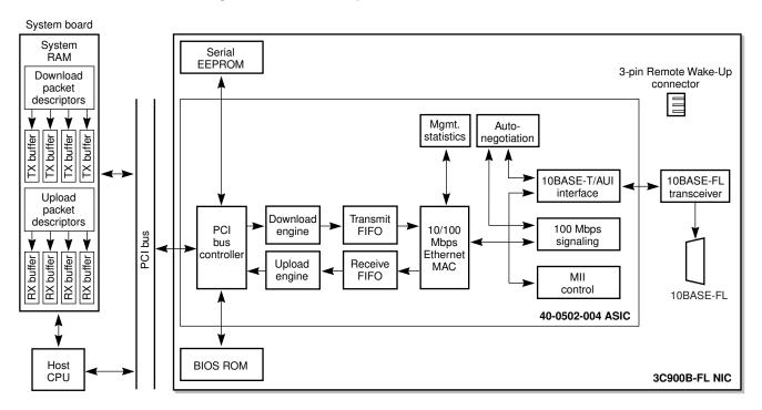
System board System Serial 3-pin Remote Wake-Up RAM EEPROM connector Download packet descriptors Mgmt. 100BASE-FX TX buffer TX buffer TX buffer statistics negotiation 10BASE-T/AUI interface Upload packet Download Transmit descriptors 100 Mbps 100BASE-FX PCI 10/100 engine **FIFO** bus Mbps signaling transceiver 입 controller Ethernet . RX buffer BX buffer BY buf RX buffer Upload Receive MAC engine FIFO MII control 40-0502-004 ASIC **BIOS ROM** Host CPU 3C905B-FX NIC
