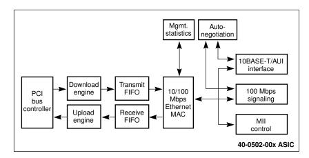
Figure 16 3C905B-TX NIC—40-0476-001 ASIC Block Diagram
