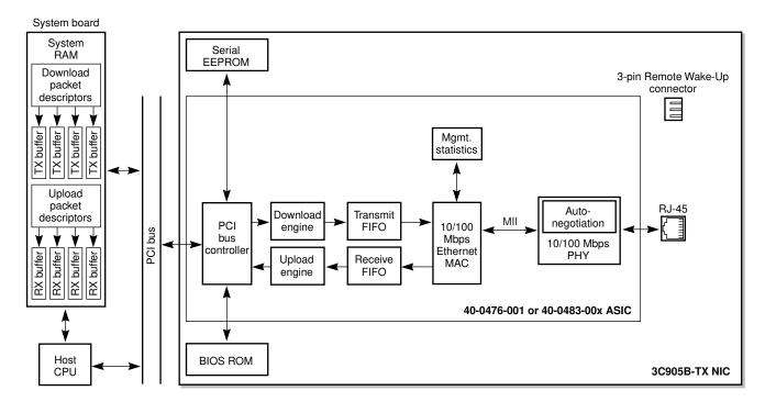
Figure 10 3C905B-TX-NM System Architecture
