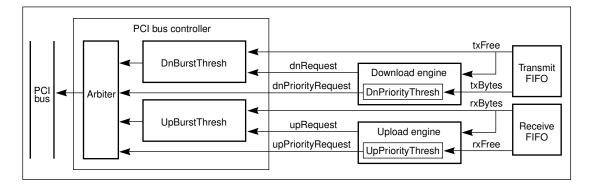
Arbitration logic (the arbiter) within the PCI bus controller block accepts bus requests from the download and upload engines.
