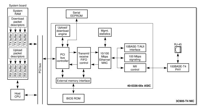
Figure 4 3C905-T4 System Architecture
